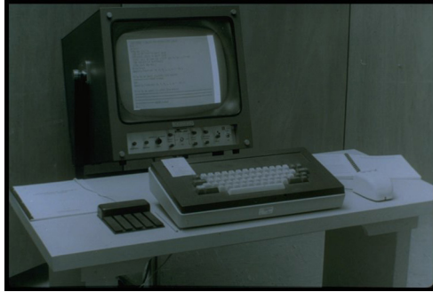
Augmentation Research Center: Prototype of an interface for computers with monitor, manual, keyset (left) and mouse (right), 1967.
