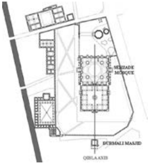
III. 8. Alignment of qibla axis's of the Sehzade mosque and Burmalı masjid
