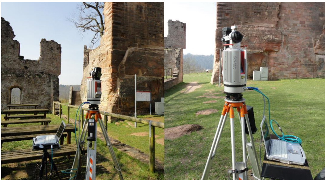
Figure 18: The Riegl VZ-400 Scanner at Castle Hohenecken on the day of the TLS recording.
