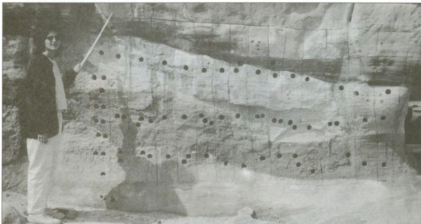
The repair mortar test field in an ancient Nabatean quarry in Petra
