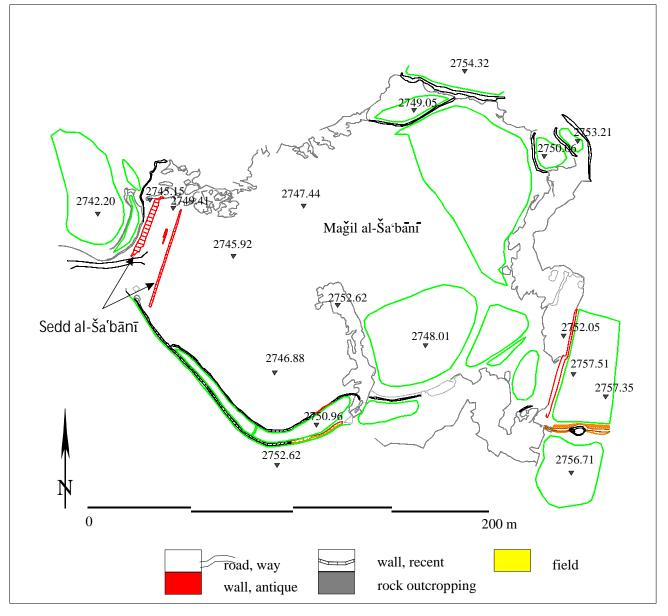
Fig. 32. Plan of the dams, Sedd al-ša'bānī, and reservoir, Ma'ğil al-ša'bānī.
