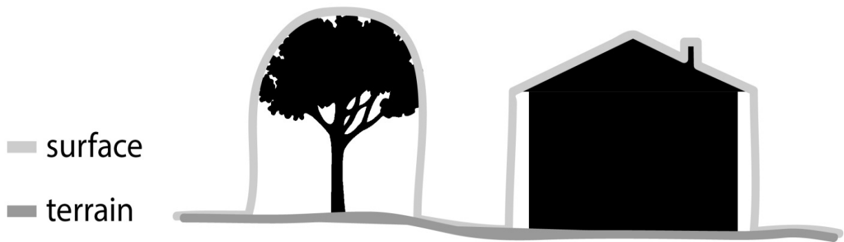
FIGURE 2: A SIMPLISTIC REPRESENTATION OF DIFFERENCE BETWEEN DSM AND DTM. SURFACE MODELS INCLUDE STRUCTURES AND CANOPIES
