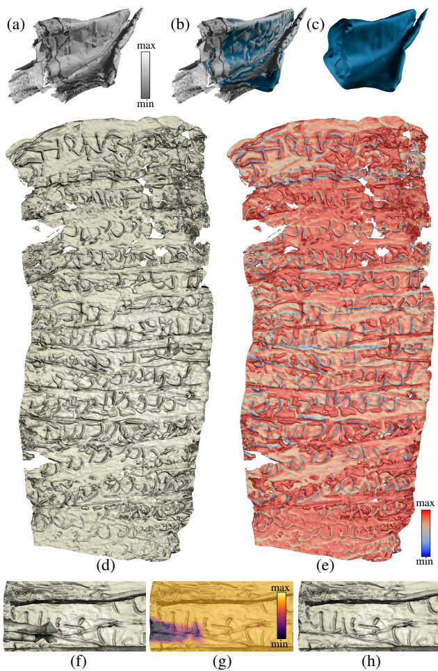
Figure 8: Silver scroll: (a) volume rendering of \mu CT image; (b) same as (a) with \mathcal{M}_{\text{curv}} ; (c) \mathcal{M}_{\text{curv}} ; (d) thin iso-surface rendering; (e) thin iso-surface rendering with distance to \mathcal{M}_{\text{curv}} color-coded (blue=behind, red=in front of \mathcal{M}_{\text{curv}} ); (f) zoom-in with occluding structure; (g) modified ray length color-coded; (h) occluding structure partially removed.
