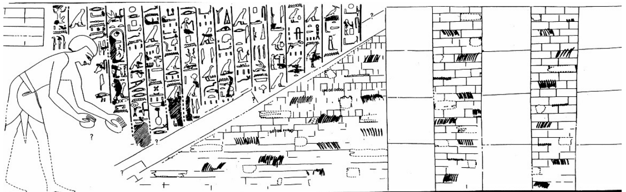
Fig. 10 Brick ramp, from the tomb of Rekhmire. 33
