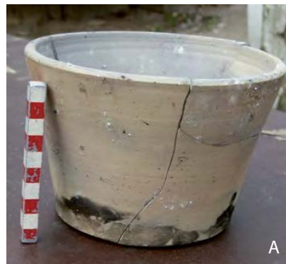
A: Reactor after deposited in a charcoal-fire by max. 722 °C.
