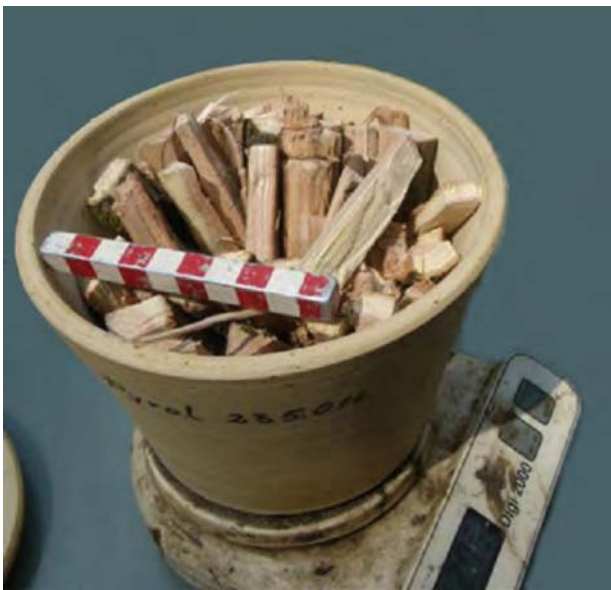
Fig. S 3-1 Conicle ceramic cylinder, fed by wood of Tamarix spec. . The cylinder at the base is closed by the perforated disc.
