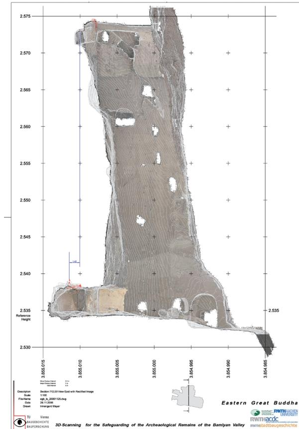
Fig. 5. Orthophoto generated from the laser scan.
