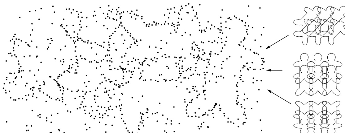
Figure 4.2: Extending the principle of sparse signal recovery (see Fig. 4.1) to the problem of 3D template matching – here in 2D for illustration – amounts to approximate the scene (left) by a small subset selected from a large collection of candidates (right panel). Again this can be achieved by convex programming.
