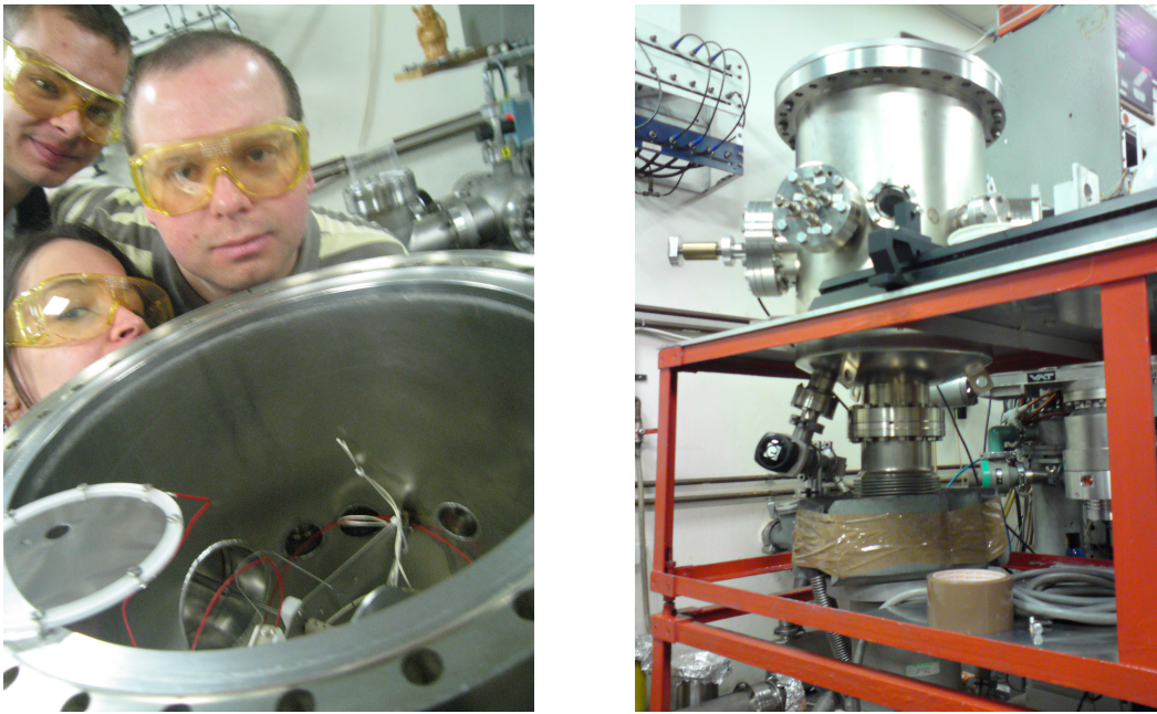
Figure 3.5.: (left) Photograph of the target chamber with some nice peoples' heads for size comparison. (right) Target chamber on its mounting with the turbo pump on bottom. Lead bricks are attached to the set up to dampen vibrations caused by the pump.
