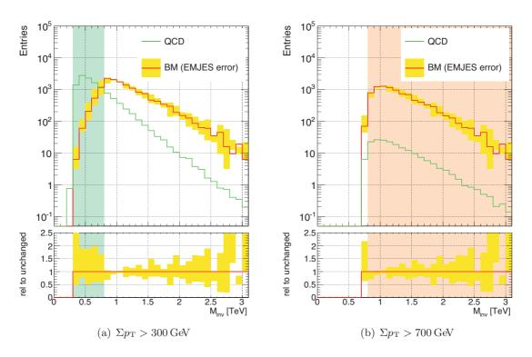
Figure 5.19.: Invariant mass distributions for the BlackMax sample with a variation of the jet energy scale. The samples are normalised to a luminosity of  $\mathcal{L}=297\,\mathrm{nb}^{-1}$ .
