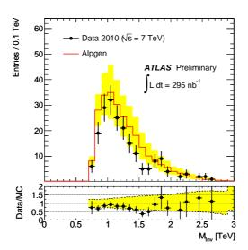
Figure 5.21.: Invariant mass distribution for an identical study with Alpgen as QCD jet production background. The shown distribution has a requirement of  $\Sigma p_{\rm T} > 700 \, {\rm GeV}$  and shows data and the Alpgen sample including all covered systematic uncertainties for a luminosity of  $\mathcal{L} = 295 \, {\rm nb}^{-1}$  [109].
