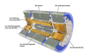
Figure 3.5.: Scheme of the ATLAS Calorimetry [40].
