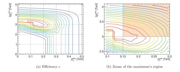
Figure 4.16.: Efficiency  $\epsilon$  as a function of  $\Sigma p_{\mathrm{T}}$  and  $p_{\mathrm{T}}^{(5)}$  for a signal sample with n=2 extra dimensions and PYTHIA plus other background processes. The contours show S on a linear scale for  $\mathcal{L}=1\,\mathrm{fb}^{-1}$  at  $\sqrt{s}=7\,\mathrm{TeV}$ . The shaded area displays the selected signal region.
