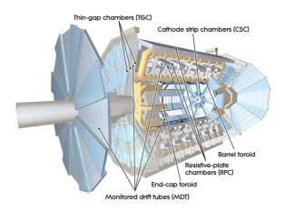
Figure 3.6.: Scheme of the ATLAS Muon System [40].
