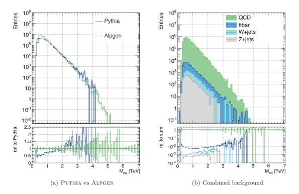
Figure 4.12.: Invariant mass distribution for  $\sqrt{s}=7\,\mathrm{TeV}$  for QCD jet production for an integrated luminosity of  $\mathcal{L}=1\,\mathrm{fb}^{-1}$  with Pythia and Alpgen (a) and for the combination of all included background processes (b). The displayed uncertainties correspond to the limited statistics of the available sample.
