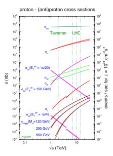
Figure 3.2.: Predictions of the total cross section ( $\sigma_{\rm tot}$ ) and cross sections for individual cross sections (left axis). Expected event rates per second at an instantaneous luminosity of  $\mathcal{L} = 10^{33} \, \mathrm{cm}^{-2} \, \mathrm{s}^{-1}$  as a function of the centre-of-mass energy  $\sqrt{s}$  [43].
