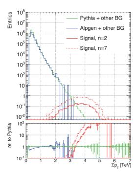
Figure 4.13.: Scalar sum of transverse momenta of all objects for background and two different signal samples with n=2(7) extra dimensions for an integrated luminosity of  $\mathcal{L}=1~\mathrm{fb^{-1}}$  at  $\sqrt{s}=7~\mathrm{TeV}$ .
