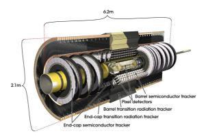
Figure 3.4.: Scheme of the ATLAS Inner Detector [40].
