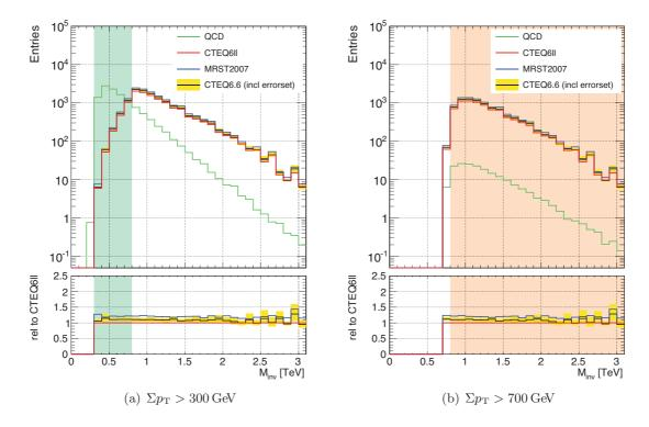
Figure 5.17.: Invariant mass distributions for the BlackMax samples with different PDF sets (CTEQ61l, CTEQ6.6, MRST2007). For the PDF set CTEQ6.6 the associated error set is used and displayed. The samples are normalised to a luminosity of  $\mathcal{L} = 297 \, \mathrm{nb}^{-1}$ .
