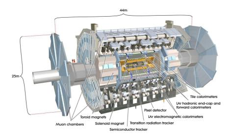
Figure 3.3.: Scheme of the ATLAS Detector [40].
