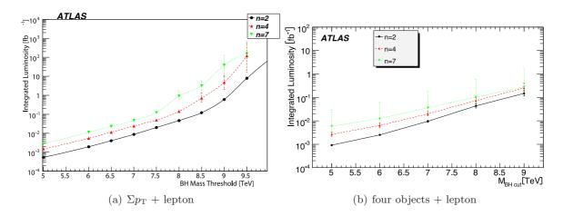
Figure 4.5.: Discovery reach for the  $\Sigma p_{\rm T}+$  lepton requirement (left) and the fourobjects + lepton requirement (right) as a function of the minimum reconstructed invariant mass for  $\sqrt{s}=14$  TeV [99].
