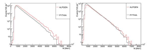
Figure 4.6.: Reconstructed invariant mass for  $\sqrt{s} = 10$  TeV for Pythia and Alpgen samples before (left) and after (right) rescaling of Alpgen at  $M_{\rm inv} = 3$  TeV [101].
