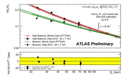
Figure 3.7.: Jet Energy Resolution for  $\sqrt{s} = 7 \text{ TeV}$ , determined with an integrated luminosity of  $6 \text{ nb}^{-1}$  [65].
