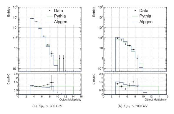
Figure 5.5.: Object multiplicity for events passing the selection criteria. The shown MC distributions are normalised to the number of data events in the control region.
