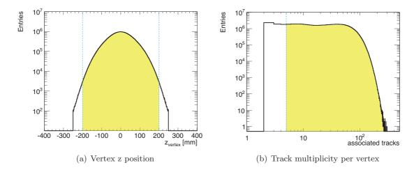
Figure 5.3.: Vertex distributions in the data sample corresponding to a luminosity of  $\mathcal{L} = 297\,\mathrm{nb}^{-1}$ . The dashed line shows the selection criterion, and the filled area the vertices passing the selection.
