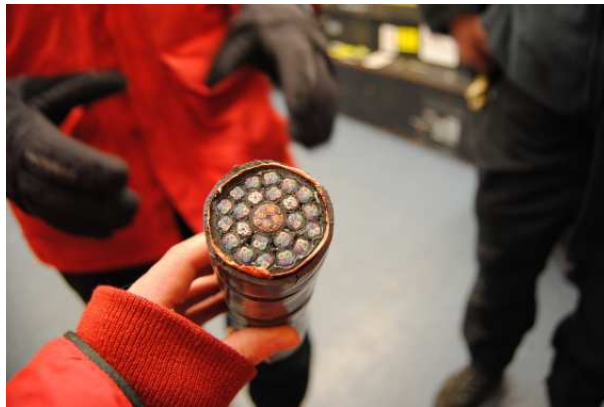
Figure 5.8.: An IceCube surface cable as used to provide the connection from the surface junction box to the IceCube laboratory (ICL) at the South Pole. Cables like this provide communication to one of the IceCube strings respectively and the two associated IceTop stations. Each string is controlled by a DOMHub computer in the ICL.
