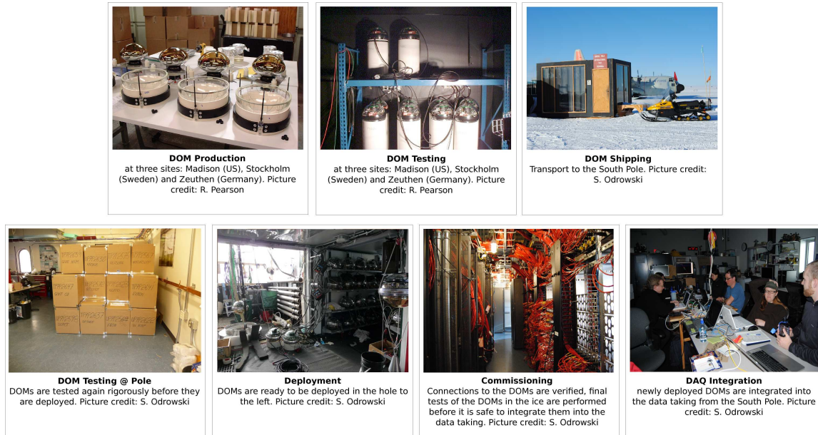
Figure 5.4.: Illustration of the steps each IceCube DOM has to pass before it forms an active part of the detector. Each DOM is tested at several stages before and after it has been deployed in the ice.
