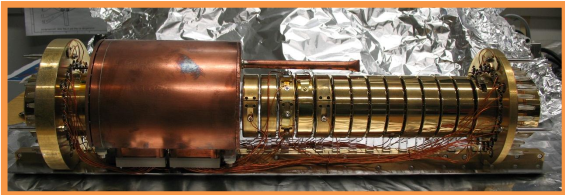
Figure 4.3: The electrode stack with mounted electronics box. Kapton coated wires connect the electrodes with the electronics box and feedthroughs to the connection system.
