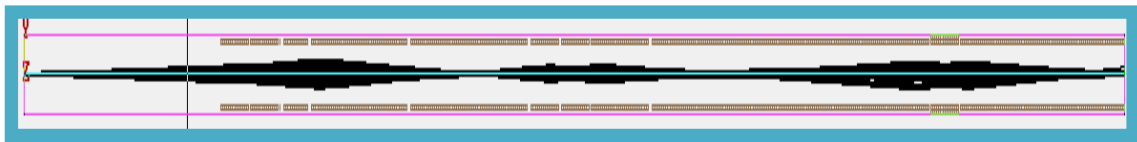
Figure 5.12: The simulated beam envelope between the ion source and the injection point. In this simulation the retardation voltage was 2.6 kV. Lens 1 was at -100 V, lens 2 at -2.3 kV and lens 3 at -1.45 kV. The injection spot has a radius of 2.2 mm. The width of the picture has been enlarged compared to its length for visual reasons.
