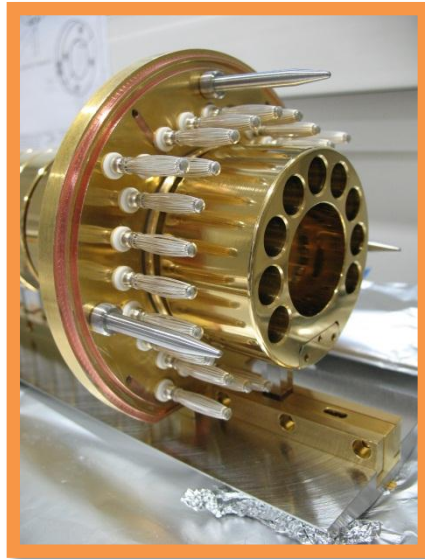
Figure 4.5: Outer electrode with feedthroughs for the electrode connections.
