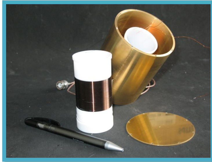
Figure 5.25: Superconducting resonator. The coil in the front is made out of superconducting NbTi. Behind is a gold plated copper resonator shield.
