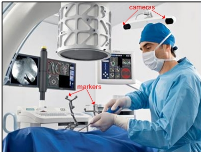
Figure 1.3.: Typical setup of an optical tracking system
