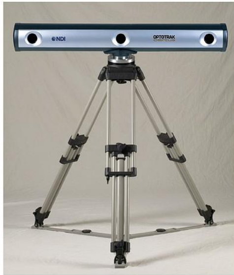
Figure 1.8.: Optotrak Certus Motion Capture System
