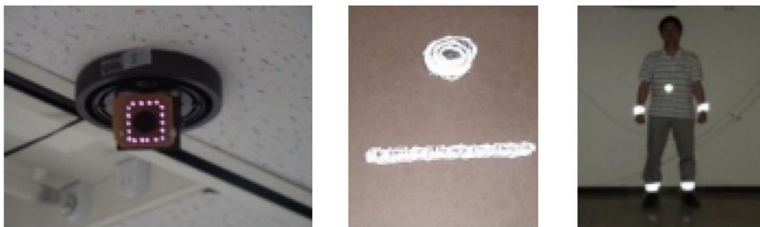
Figure 1.10.: Camera and markers used in POSTTRACK
