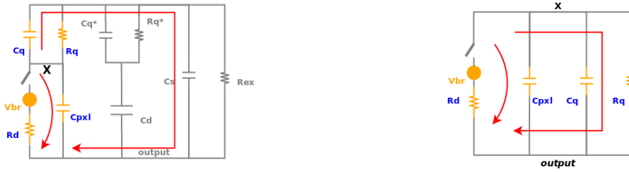
Figure 2.38: Circuit for decay constant calculation: AC model (left) and simplified model (right)
