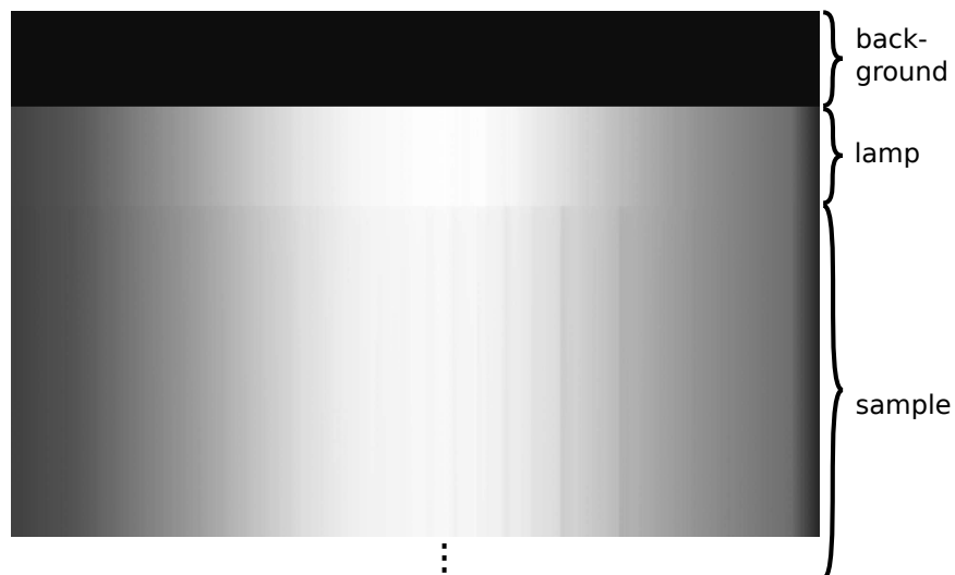
Figure 5.1.: Example of a UV spectroscopy raw data image. Each line contains 1 spectrum. For better illustration, the image is cropped considerably at the bottom as well as slightly cropped on the left and right side. The first 200 spectra correspond to dark spectra, followed by 200 lines of lamp spectra without any tracers.
