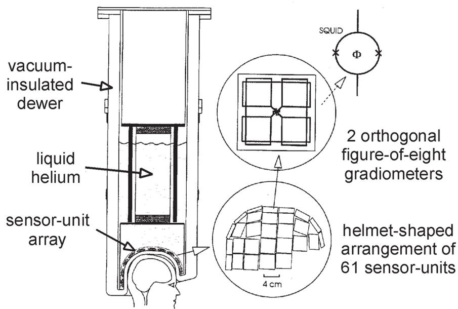
Figure 3.6: *The Neuromag-122 channel whole head MEG system. At each of 61 sensor positions in the head-shaped arrangement of this system, two figure-of-eight gradiometers with orthogonal orientations measure the planar gradients of the magnetic flux emerging from the head.*
