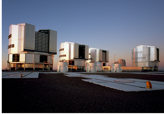
FIGURE 1.7: The ground-base Very Large Telescope (VLT). The four main VLT units can be seen, as well the four auxiliary telescopes. The High Acuity Wide field K-band Imager of VLT (VLT/HAWK-1) is one of the best ground-based instruments to provides deep wide-area high-resolution near-infrared images. The Paranal platform photographed in January 2007. Credit:ESO/H.H.Heyer.
