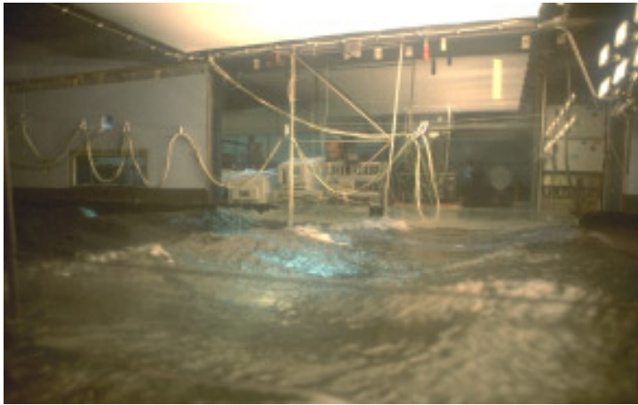
Figure 5: Wave slope visualization system in operation at high wind speeds in the large wind/wave flume of the IMST, University of Marseille, France. The system is viewed through one of the large glass windows of the facility. In the upper right corner, some of the lamps can be seen used to illuminate the large screen. (For color figure, see Plate 5.)
