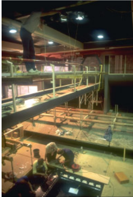
Figure 2: Close to the beach and air-flow return section, the 10 m wide corridor section of the Delft wind wave facility (see Figure 1) opens to a 30 m wide and 5.5 m high end section. Instruments can directly be built into the bottom of the facility, replacing 2 \times 2 \text{ m}^2 large and 0.2 m high concrete plates. With a traveling bridge instruments can be mounted at the ceiling. (For color figure, see Plate 15.)
