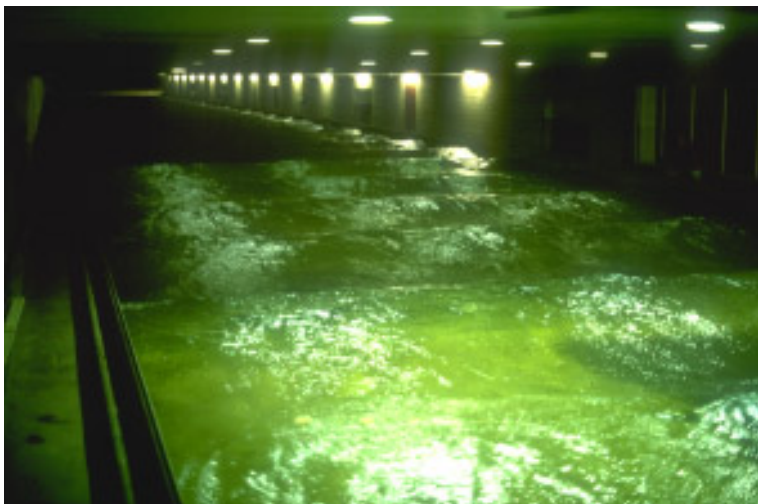
Figure 1: A view from the sidewalk of the Delft wind/wave flume at about 90 m fetch in downwind direction while the facility is in operation at 12 m/s wind speed. The water channel is 8 m wide. (For color figure, see Plate 14.)
