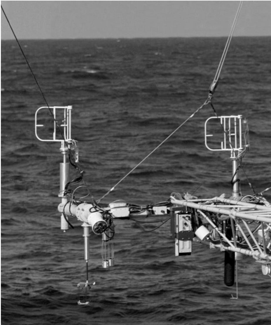
Figure 1: Sensors on the MPN boom in ASGASEX. Upper left and right, BIO and KNMI sonic anemometers are separated by 2 m. KNMI IFM water vapour and CO 2 sensor is attached just behind (to right of) KNMI sonic; BIO Lyman-alpha humidity meter and microbead thermistor are just behind base of BIO sonic. TNO sonic anemometer is at lower left, with two Advanet IR water vapour and CO 2 sensors just to the right and above it. KNMI pressure anemometer is at lower right. Boom is on west side of MPN; camera is pointing towards northwest.
