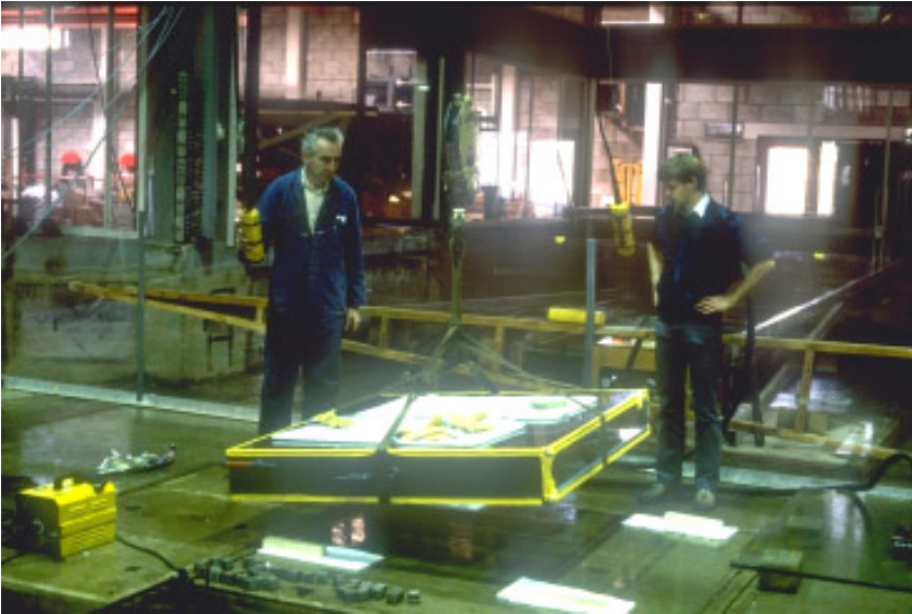
Figure 3: Heavy equipment can easily be moved around in the Delft wind/wave flume by a travelling crane. Here it is shown how the illumination unit of wave slope imaging is lowered to the bottom of the empty facility. (For color figure, see Plate 16.)
