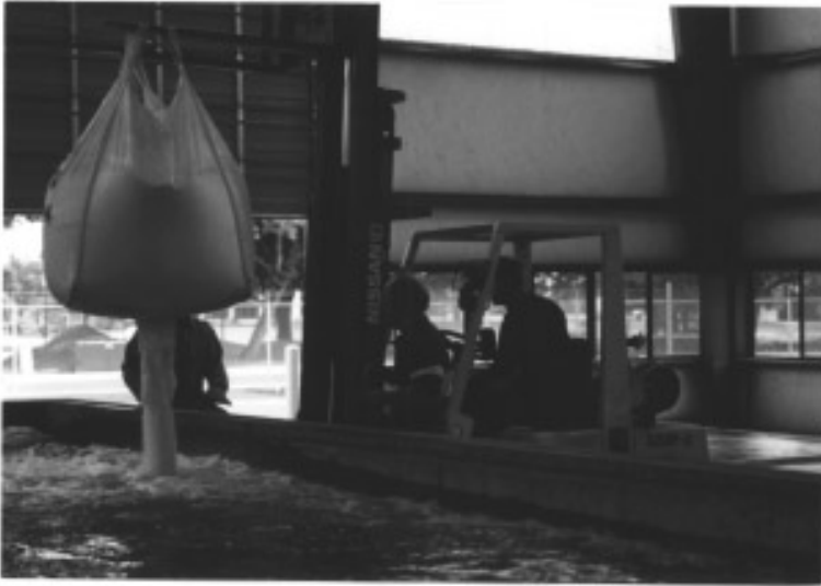
Figure 2: A photograph of the salt mixing section with a one ton bag of salt being added.
