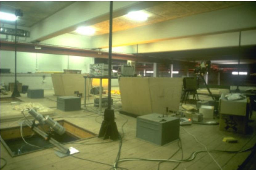
Figure 4: View of the instrumentation deck on the top of facility in the last part of the corridor section from 75–90 m fetch. Through several 1 \times 1 \text{ m}^2 large openings, instruments can be mounted to make measurements from above. (For color figure, see Plate 17.)
