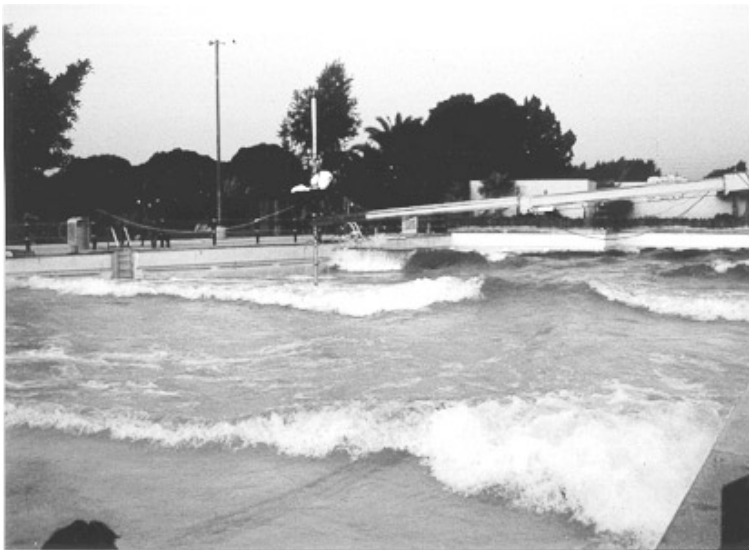
Figure 2: Photograph of a typical 1.2-m high plunging breaking wave generated by the Roller Pattern. The crane arm holding the radiometer is seen in the center of the picture.
