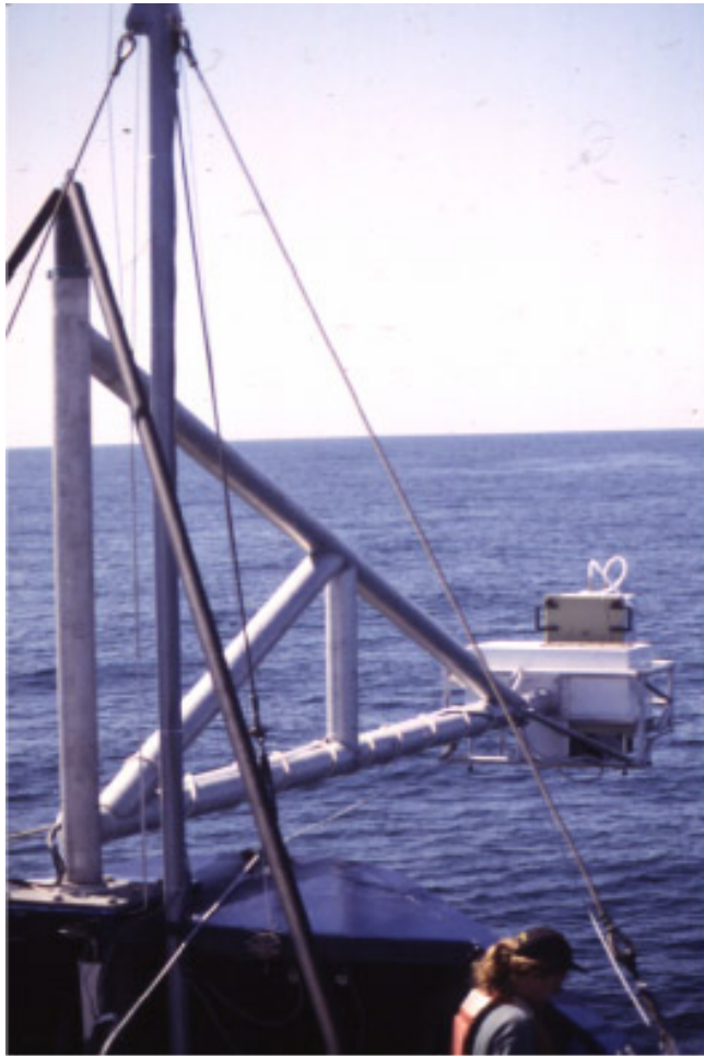
Figure 2: The Controlled Heat Flux boom on the R/V New Horizon during the April/May 1995 NSF CoOP cruise off Monterey Bay.
