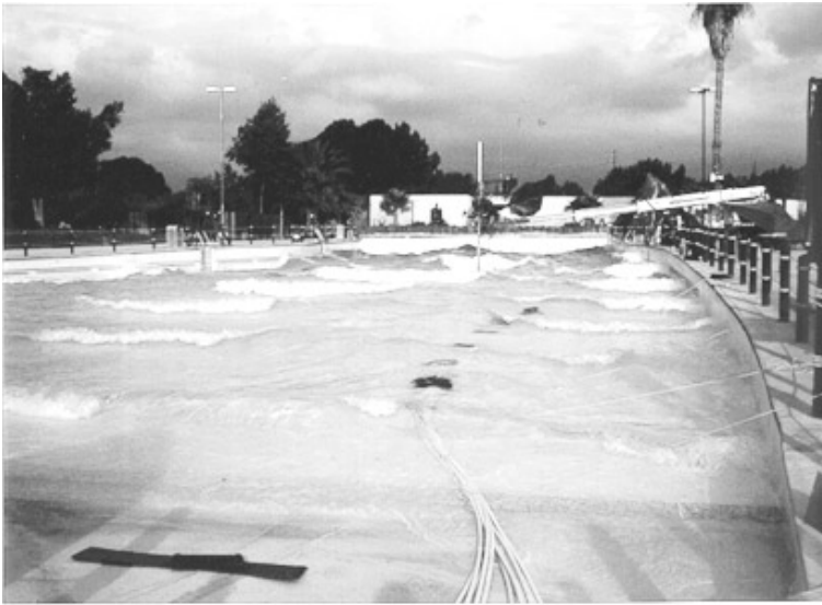
Figure 3: Photograph of typical 0.9-m high spilling breaking waves generated by the Diamond Pattern. The crane arm holding the radiometer is seen in the center of the picture.
