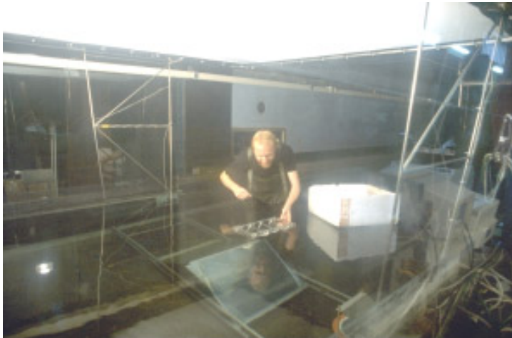
Figure 4: Wave slope visualization system used by the author in the large wind/wave flume of the IMST, University of Marseille. A large screen close to the ceiling is illuminated from aside by two rows of lamps (see Figure 5) to produce an intensity wedge in wind direction. In this way, the along-wind wave slope can be made visible. Through the plane water surface, the submerged optical parts can be seen. In order to increase the distance of the camera to the water surface, the optical path is folded two times by mirrors. Slope calibration is — as shown in the figure — performed by using an artificial wave consisting of a Perspex foil bent by a frame into a sinusoidal shape. The whole system is mounted onto a carriage so that it can be moved through the facility. (For color figure, see Plate 4.)
