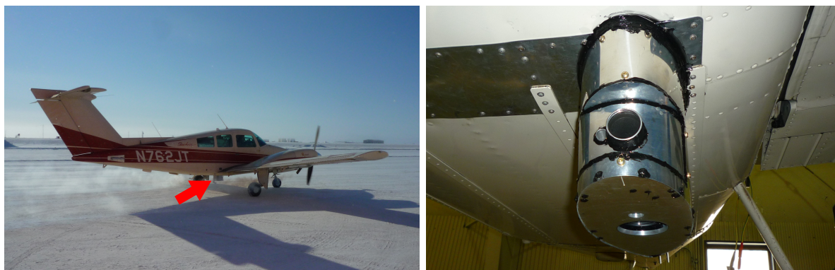
Figure 3.60.: Installation of the HAIDI system on the Beechcraft Model 76 Duchess from Purdue University. The picture on the right hand side shows the aircraft shortly before takeoff, the box that contains the entrance optics for nadir scanner and forward-looking telescope is marked by the red arrow. On the right hand side a closer view of the aircraft's lower shell is shown, including the aerodynamic fairing with viewports for both instruments and additional webcams. The box is connected to the spectrographs and CCD cameras inside the aircraft via a fiber optics cable going through the fuselage.
