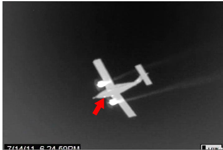
Figure 3.62.: Single frame from a CO-sensitive infrared video camera, showing ALAR in flight. Exhaust gases and heat sources like engines are shown in white color. As can be seen, the exhaust from the two engines disperses laterally very little over the length of the aircraft and could therefore not affect the measurements. Also the exhaust from the heater (red arrow) proved to be unproblematic, since it is located on the opposite side of the aircraft's lower shell and no exhaust plume is visible. Picture courtesy of Brian Stirm.
