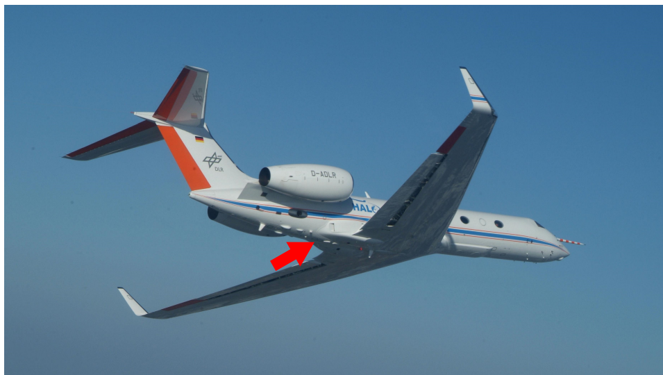
Figure 3.66.: Picture showing HALO in flight (DLR, 2013a). The two apertures ApB-8 and ApB-9, which are the preferred position for the entrance optics of the HAIDI system, are marked by the red arrow.
