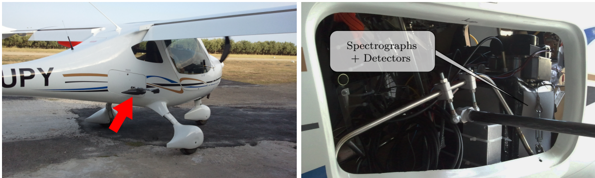
Figure 3.58.: Installation of the HAIDI system on board of an ultralight aircraft (Flight Design CTLS) during the measurements on Sicily, Italy. Spectrographs, CCD cameras, netbooks and a battery pack were stored inside the baggage compartment (picture on the right) while the entrance optics is mounted outside the aircraft at a carbon fiber extension arm (left picture).
