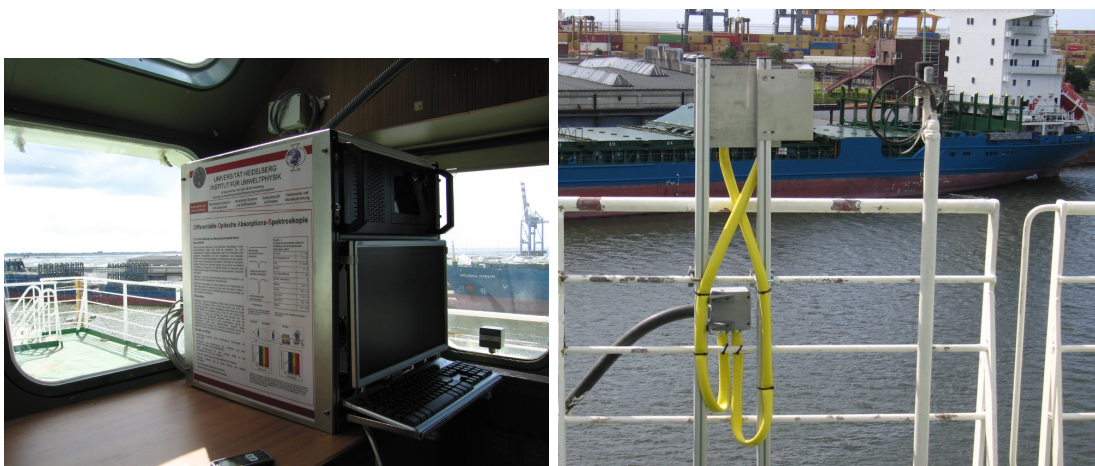
Figure 4.1.: The permanent MAX-DOAS instrument on R/V Polarstern. The spectrometer is located inside, the inclination corrected telescope unit at the portside railing.
