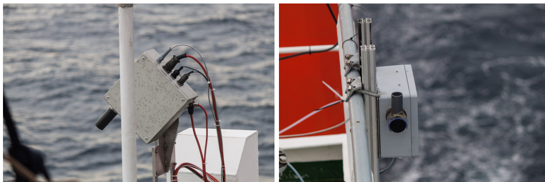
Figure B.2.: The MAX-DOAS telescopes from Bremen and Heidelberg, looking into different directions, Bremen to starboard side, Heidelberg to portside.
