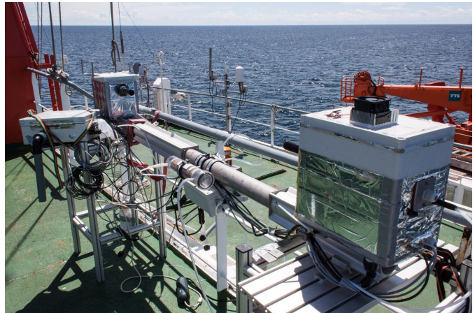
Figure 4.4.: The open-path CE-DOAS setup during SHIVA on R/V Sonne in November 2011.
