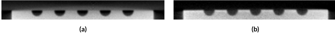
Figure 3.8: Artifacts at the top of the reconstructed cube. In the FDK reconstructed object (b) cone beam artifacts occur at the top of the cube. When using the Katsevich's FBP algorithm no cone beam artifacts are visible (a).
