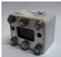
Figure 2.2 Measurement chamber for XRR at solid-liquid interface. The liquid cell consisted of a self-made Teflon main body with Kapton windows. The silicon wafer was inserted prior the membrane preparation.
