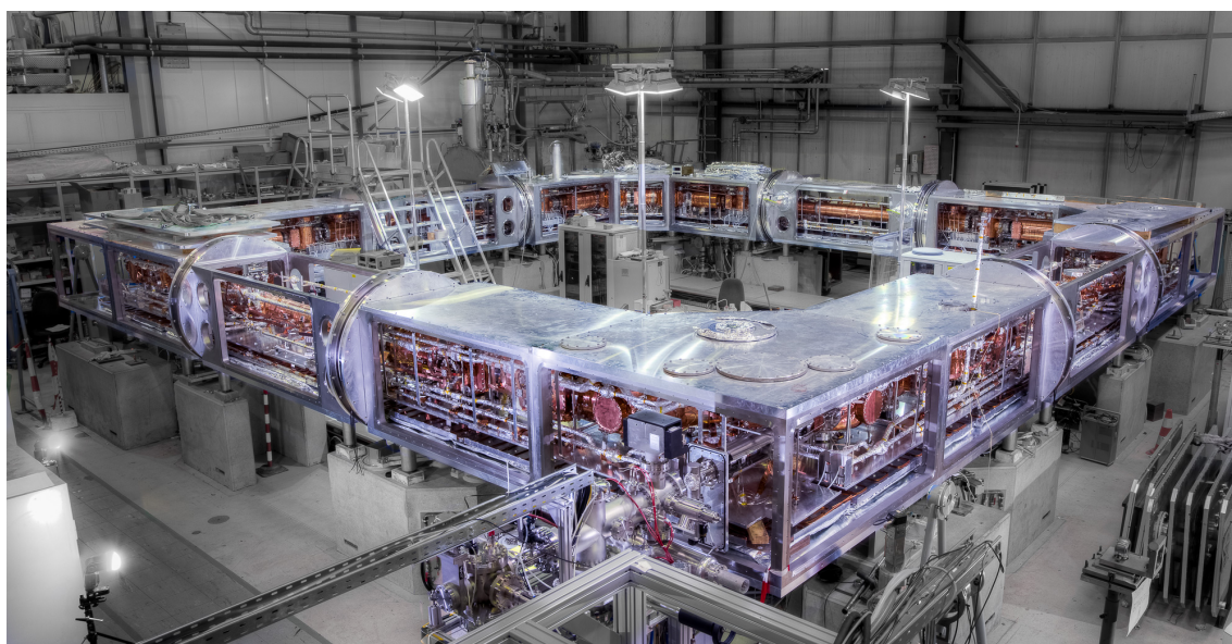
Figure 3.3: Photograph of the Cryogenic Storage Ring just before the first commissioning at room-temperature in spring 2014. The outer isolation vacuum chamber is still open. The beam-guiding chamber is wrapped in copper. The isolation vacuum chamber was closed before the storage operation.
