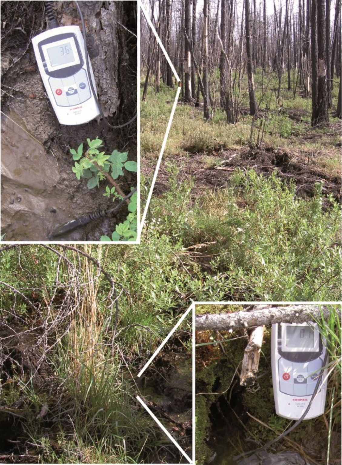
Figure 22: Upslope view of a 55 m hillslope section with observed preferential sub-surface flow and return flow; inserted photographs show details and measured water temperature.
