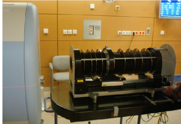
Figure 4.3: The PEAKFINDER T41030 Water Column from PTW was used to measure the WET of the targets. Reprinted from Sánchez Parcerisa 2012.
