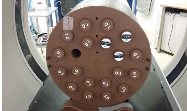
Figure 5.7: The configuration of the density plugs used in the tests of the heterogeneous setup of the cheese phantom.
