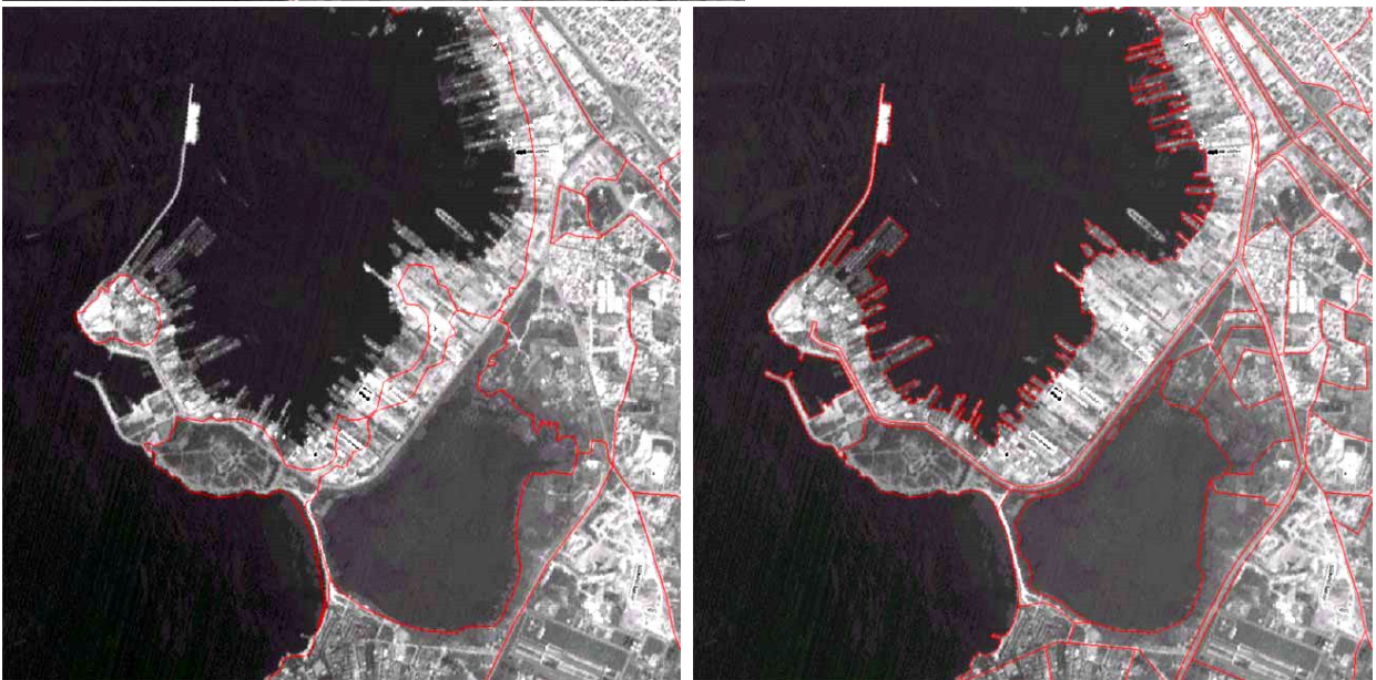
Figures 129 and 130: The images below are IRS-Pan of the year 2000. The same areas than before with the land use boundaries from 1945 (left) and from 2000 (right) where port areas were constructed.
