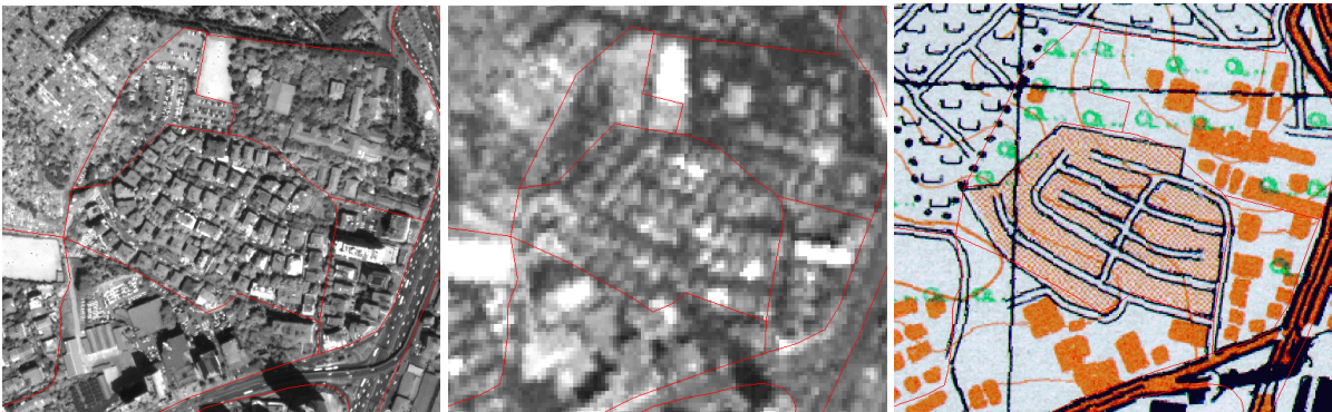
Figure 79: left = IKONOS pan, middle = IRS-D pan, right = Map 1:25k : shown is residential surface with class 1.1.1.1
