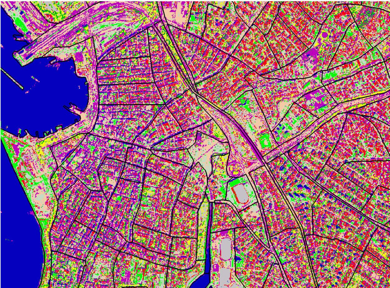
Figure 76: Example of a classified IKONOS MS-satellite image, using 4 bands, with the overlaid manually digitised land-use pattern
