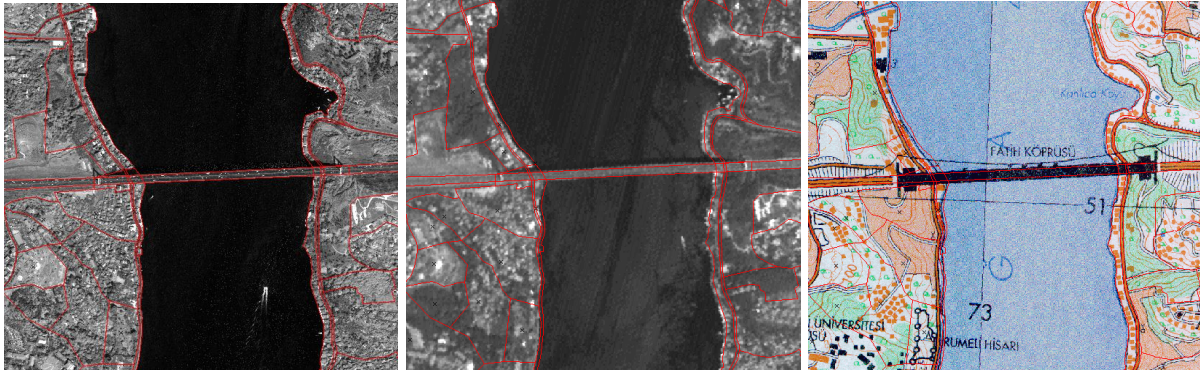
Figure 86: left = IKONOS pan, middle = IRS-D pan, right = Map 1:25k : shown is the highway cross the northern Bosphorus-Bridge; class 1.2.2.1
