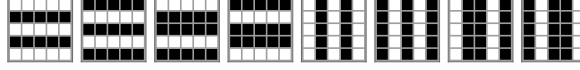
Figure 4.5. - 8 binary filter masks for computing the feature vectors corresponding to each pixel. After correlating an input image, the resulting values were encoded for each pixel by stacking corresponding unit-vectors. This resulted in feature vectors f^i \in \mathbb{R}^{97} with a large number of degrees of freedom for learning. In view of the images from Fig. 4.4.
