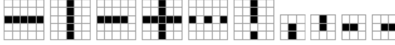
Figure 4.10. - We used 10 binary filter masks for computing feature vectors. After correlating an input image with each of the filters masks, we use neighboring feature vectors for computing Gaussian kernels, in order defining the pairwise features as in (4.103).
