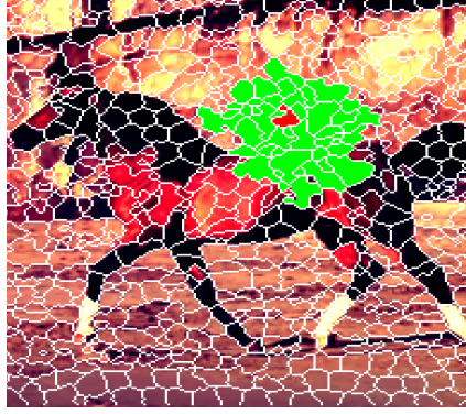
Figure 4.13. - A sample horse image from the Weizmann horse dataset [BU08] segmented into SLIC superpixels [ASS + 12]. The white lines are the border lines of each superpixel. We colored in red the center superpixel for which we illustrate its three layer neighboring superpixels in green.
