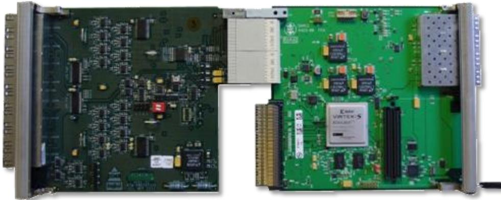
Figure 4.1.: The DESY DAMC2 board and the C&C RTM connected [43].
