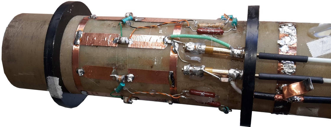
Figure 3.1: Photograph of the 8-legged low-pass Birdcage coil without the shield.
