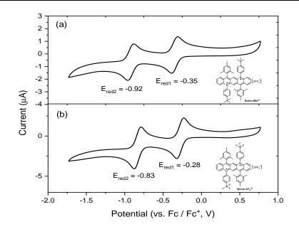
**Figure 36.** CVs of a) **Quino-tBu**<sup>2+</sup> and b) **Quino-CF**<sub>3</sub><sup>2+</sup> using a gold working electrode, a platinum/titanium wire auxiliary electrode, and a silver wire reference electrode in degassed 0.1 M NBu<sub>4</sub>PF<sub>6</sub> DCM solution. The electrode potential was externally calibrated by Fc/Fc<sup>+</sup> couple. Adapted with permission of ref. 120 © 2020, Wiley-VCH.
