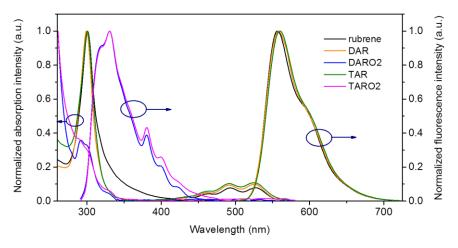
**Figure 15**. Normalized absorption and emission spectra of rubrene and designed compounds measured in DCM. Reproduced with permission of ref. 77 © 2018, the Royal Society of Chemistry.
