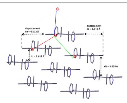
**Figure 18**. Illustration of the lattice parameters within **ab** layer of **DAR** crystal. The  $\pi$ - $\pi$  stacking distances along **a** and **b** direction are estimated to be around 3.6 Å and 5.6 Å respectively; the long-axis displacements of adjacent molecule along **a** and **b** direction are estimated to be around 6.1 Å and 4.4 Å respectively. Reproduced with permission of ref. 77 © 2018, the Royal Society of Chemistry.
