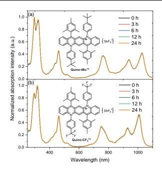
**Figure 33**. Time-dependent absorption spectra of a) **Quino-tBu**<sup>++</sup> and b) **Quino-CF**<sub>3</sub><sup>++</sup> measured in DCM under ambient conditions. Adapted with permission of ref. 120 © 2020, Wiley-VCH.
