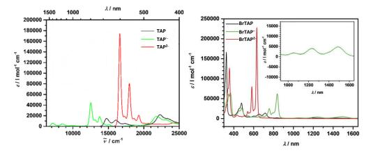
**Figure 12.** UV-vis spectra of the neutral (black), singly negatively charged (green), and doubly negatively charged (red) of **TAP** (left) and **Br<sub>4</sub>TAP** (right). Left panel adapted with permission of ref. 71 © 2017, American Chemical Society, and right panel adapted with permission of ref. 72 © 2018, Wiley-VCH.
