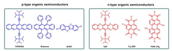
**Figure 3.** Representative p- and n-type organic semiconductors (**TIPSPEN**,<sup>[14]</sup> **Rubrene**,<sup>[11]</sup> **BTBT**,<sup>[15]</sup> **TAP**,<sup>[16]</sup> **Cl**<sub>2</sub>-**NDI**,<sup>[17]</sup> and **PDIF-CN**<sub>2</sub><sup>[18]</sup>).
