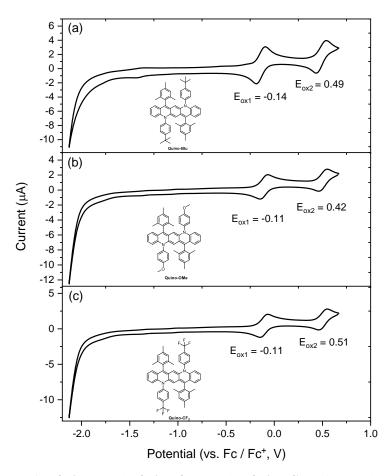
**Figure 34**. CVs of a) **Quino-tBu**, b) **Quino-OMe**, and c) **Quino-CF**<sub>3</sub> using a gold working electrode, a platinum/titanium wire auxiliary electrode, and a silver wire reference electrode in degassed 0.1 M NBu<sub>4</sub>PF<sub>6</sub> DCM solution. The electrode potential was externally calibrated by  $Fc/Fc^+$  couple. Adapted with permission of ref. 120 © 2020, Wiley-VCH.
