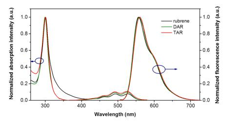
**Figure 14**. Normalized absorption and emission spectra of rubrene, **DAR** and **TAR** measured in DCM. Reproduced with permission of ref. 77 © 2018, the Royal Society of Chemistry.
