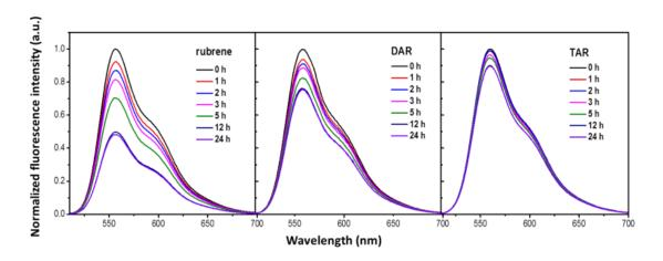
**Figure 16**. Normalized time-dependent emission spectra of rubrene, **DAR**, and **TAR** measured in DCM. Reproduced with permission of ref. 77 © 2018, the Royal Society of Chemistry.
