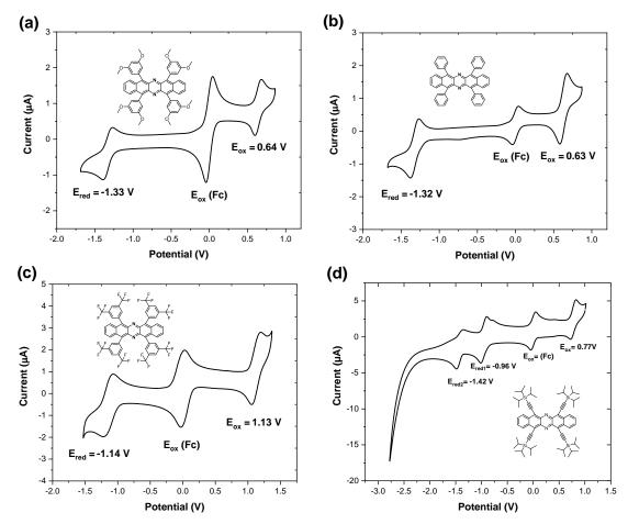
CVs of a) **3a**, b) **3b**, c) **3c**, and d) **3d** with ferrocene:
