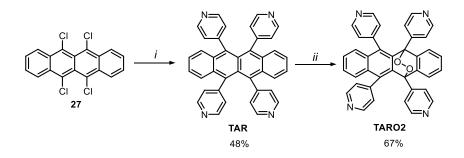
**Scheme 14.** Synthetic route to **TAR**. *i*) 4-Pyridinylboronic acid; tris(dibenzylideneacetone) dipalladium(0) (Pd<sub>2</sub>dba<sub>3</sub>), 2-dicyclohexylphosphino-2',4',6'-triisopropyl-biphenyl (Xphos), K<sub>3</sub>PO<sub>4</sub>, 1,4-dioxane, 100 °C, 72 h; *ii*) air, DCM, r.t., 5 d. Reproduced with permission of ref. 77 © 2018, the Royal Society of Chemistry.
