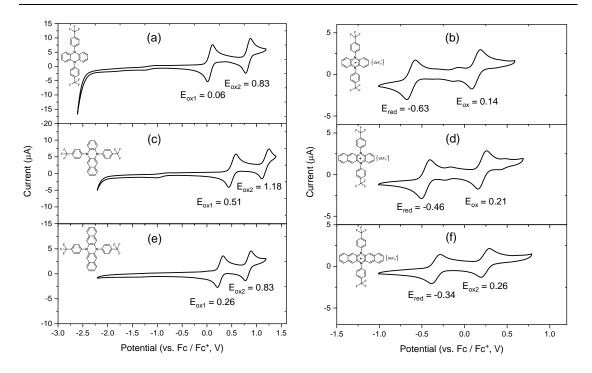
**Figure 45**. CVs of a) **PNZ**; b) **PNZ**<sup>+</sup>; c) **BPNZ**; d) **BPNZ**<sup>+</sup>; e) **DPNZ**; f) **DPNZ**<sup>+</sup> using a glass-carbon working electrode, a platinum/titanium wire auxiliary electrode, and a silver wire reference electrode in degassed 0.1 M NBu<sub>4</sub>PF<sub>6</sub> DCM solution. The electrode potential was externally calibrated by  $Fc/Fc^+$  couple.
