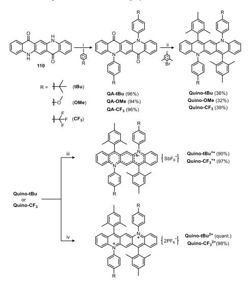
**Scheme 18.** Synthetic details towards nitrogen-embeded quinodial pentacenes and their corresponding radical cations and dications. i) 2,2,6,6-Tetramethyl-3,5-heptanedione,  $K_2CO_3$ , CuI, DMF, 146 °C, 36 h; ii) (a) *n*-BuLi, THF, -78 °C to r.t., 12 h; (b) SnCl<sub>2</sub>, THF, r.t. 1 h iii) AgSbF<sub>6</sub>, DCM, r.t., 12 h; iv) NO<sup>+</sup>PF<sub>6</sub>, DCM, r.t., 12 h. Adapted with permission of ref. 120 © 2020, Wiley-VCH.
