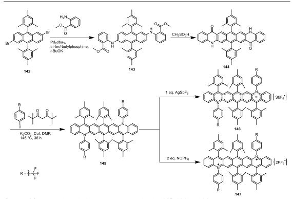
Scheme 24. Proposed synthetic route to target molecules 145, 146, and 147.
