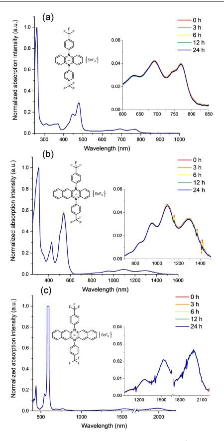
Figure 44. Normalized time-dependent absorption spectra of a)  $PNZ^+$ ; b)  $BPNZ^+$ ; c)  $DPNZ^+$  measured in DCM.
