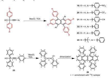
Scheme 4. Synthesis of rubrene analogues using a one-pot approach (19-22,<sup>[46]</sup> 23-24,<sup>[43]</sup> and 26<sup>[48]</sup>).
