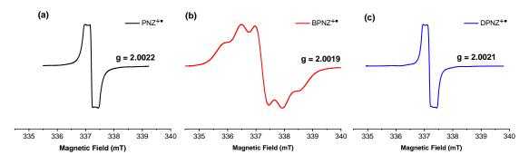
Figure 41. EPR spectra of (a) PNZ<sup>+</sup>, (b) BPNZ<sup>+</sup>, and (c) DPNZ<sup>+</sup> recorded in DCM under ambient conditions.
