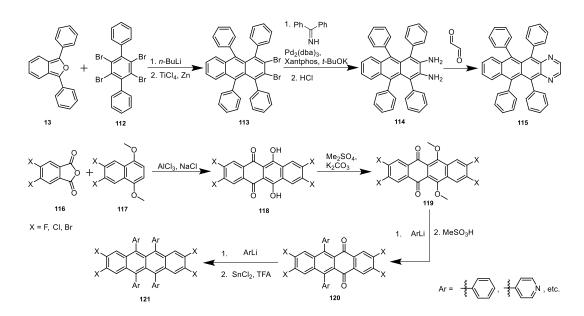
Scheme 21. Proposed synthetic route to target molecules 115 and 121.
