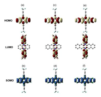
**Figure 47**. HOMOs and LUMOs (top) of a) **PNZ**; c) **BPNZ**; e) **DPNZ** calculated at DFT/B3LYP/6-311++G\*\*//DFT/B3LYP/6-311+G\*\* level of theory. Spin-density distributions (bottom) of b) **PNZ**<sup>+</sup>; d) **BPNZ**<sup>+</sup>; f) **DPNZ**<sup>+</sup> calculated at DFT/UB3LYP/6-311++G\*\* //DFT/B3LYP/6-311+G\*\* level of theory.<sup>[135]</sup>
