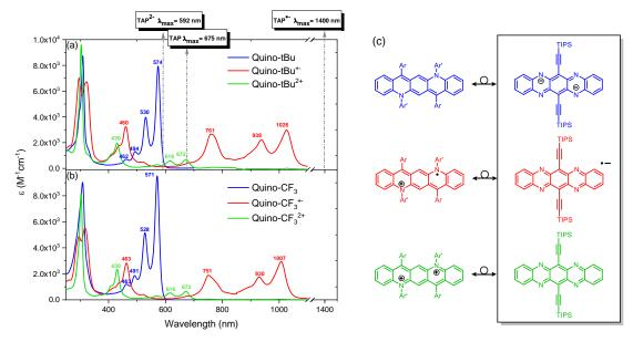
**Figure 30.** Absorption spectra of a) **Quino-tBu**, **Quino-tBu**<sup>+</sup>, and **Quino-tBu**<sup>2+</sup> (dotted arrows: maximum absorptions of TAP, TAP<sup>-</sup>, and TAP<sup>2-</sup>); b) **Quino-CF<sub>3</sub>**, **Quino-CF<sub>3</sub>**, and **Quino-CF<sub>3</sub>**, where the second second
