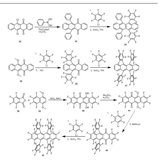
Scheme 6. Synthesis of fluoro-substituted rubrenes 34,<sup>[50]</sup> 37,<sup>[50]</sup> and 43<sup>[51]</sup>.
