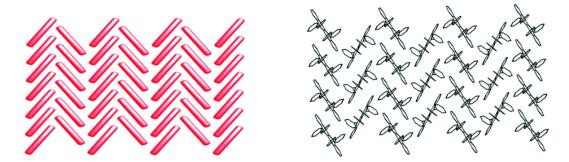
**Figure 5**. Herringbone packing motif of orthorhombic rubrene crystals. Adapted with permission from ref. 39 © 2018, American Chemical Society.
