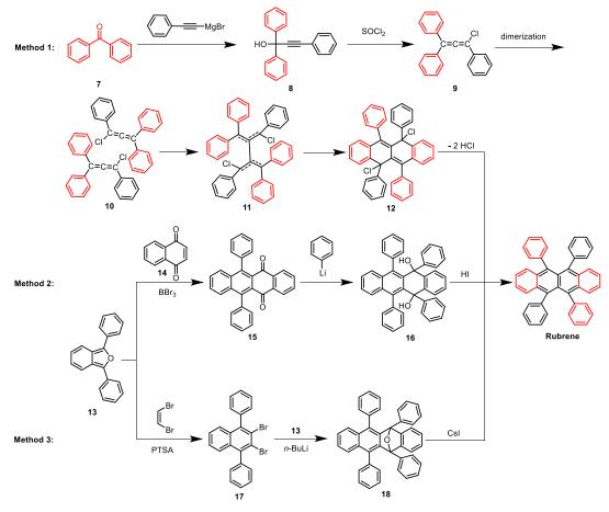
**Scheme 3.** Three synthetic routes to rubrene (method 1,<sup>[43]</sup> method 2,<sup>[44]</sup> and method 3<sup>[44]</sup>).
