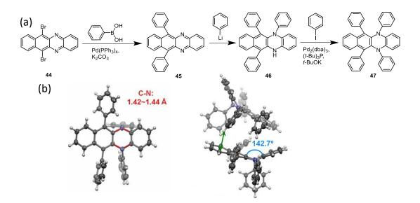
**Figure 10.** (a) Synthesis and (b) single crystal structures of **50**. Adapted with permission of ref. 52 © 2017, Wiley-VCH.
