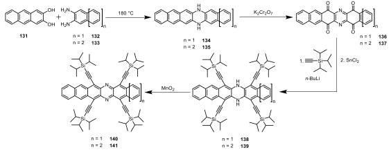
Scheme 23. Proposed synthetic route to target molecules 140 and 141.
