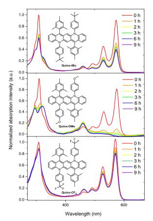
Figure 32. Time-dependent absorption spectra of Quino-tBu, Quino-OMe, and Quino-CF<sub>3</sub> measured in DCM under ambient conditions. Adapted with permission of ref. 120  $\otimes$  2020, Wiley-VCH.
