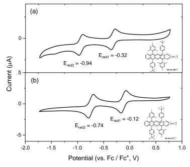
**Figure 35.** CVs of a) **Quino-tBu<sup>+</sup>** and b) **Quino-CF<sub>3</sub><sup>+</sup>** using a gold working electrode, a platinum/titanium wire auxiliary electrode, and a silver wire reference electrode in degassed 0.1 M NBu<sub>4</sub>PF<sub>6</sub> DCM solution. The electrode potential was externally calibrated by Fc/Fc<sup>+</sup> couple. Adapted with permission of ref. 120 © 2020, Wiley-VCH.
