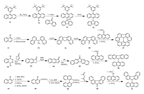
Scheme 9. Synthesis of fluorenyl-based radicals 76,<sup>[68]</sup> 81,<sup>[69]</sup> 86,<sup>[69]</sup> and 91<sup>[69]</sup>.
