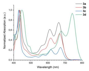
**Figure 22.** Normalized absorption spectra of **3a-3d** measured in DCM. Adapted with permission of ref. 97 © 2020, Wiley-VCH.
