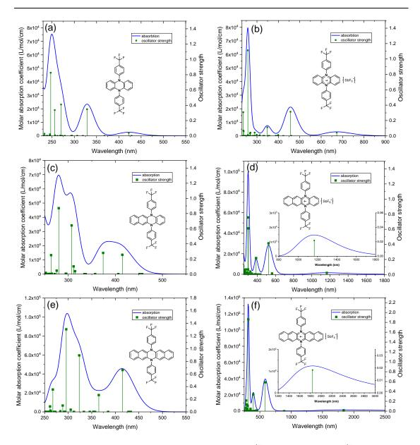
**Figure 43.** Simulated absorption spectra of a) **PNZ**; b) **PNZ**<sup>+</sup>; c) **BPNZ**; d) **BPNZ**<sup>+</sup>; e) **DPNZ**; f) **DPNZ**<sup>+</sup> calculated with Gaussian 16 at B3LYP/6-311++G\*\*//DFT/B3LYP/6-311+G\*\*/DCM level of theory.<sup>[135]</sup> The spectra were broadened using Gaussian functions with a full-width at half maximum of 0.2 eV.
