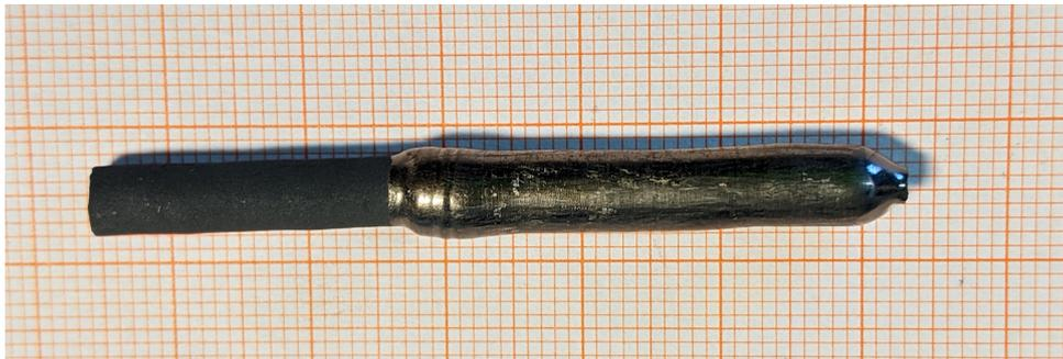
**Figure D.1.** Picture showing the optical floating-zone grown  $\text{La}_4\text{Ni}_3\text{O}_{10}$  boule at 20 bar oxygen pressure.
