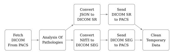
Figure 4.19: Processing pipeline for the extraction of lung pathologies.
