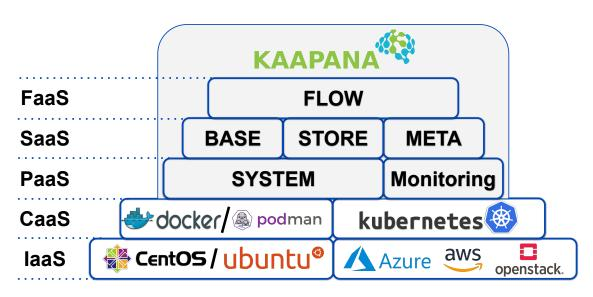
Figure 3.2: Kaapana's technology stack with its different layers.
