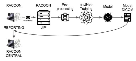
Figure 4.36: Processing pipeline for the nnUNet-training for the RACOON use case.
