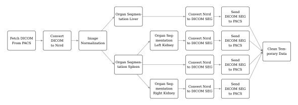
Figure 4.10: Processing pipeline for the 3D-SSM based organ segmentation.
