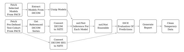
Figure 4.39: Processing pipeline for the ensembling of models.
