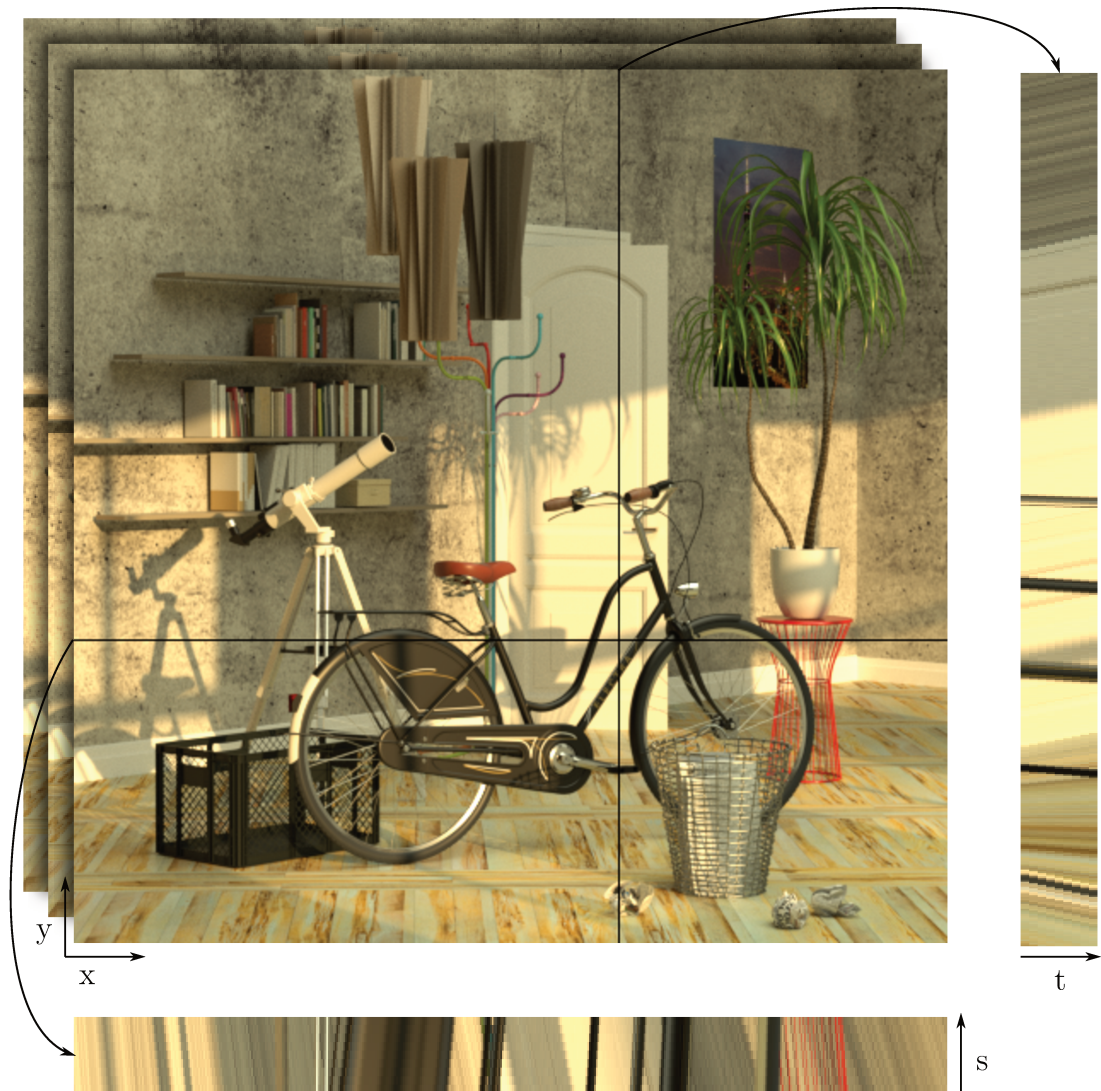
Figure 5.5: Epipolar Plane Images (EPIs) are extracted from a linear 3D subset of the 4D light field, by extracting all rows (for a horizontal subset) and stacking them together, shown at the bottom. For the vertical stack the same is done with columns. Because the apparent motion of scene points between the different viewpoints depends on the depth of the point within the scene, the orientation of features in the EPI encodes the depth of the respective points. Note that the EPI shown here is pre-shifted so a disparity of 0 is not at infinity but rather within the scene, hence disparities may also be negative.
