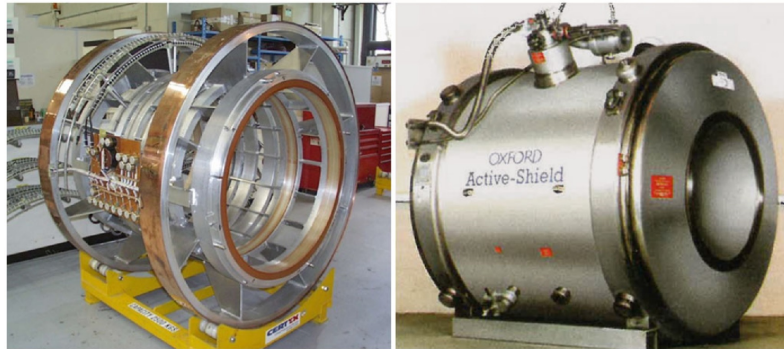
Figure 2.2: The superconducting coil required for generating the magnetic main field for MRI is shown on the left; the right shows the cryogenic vessel containing helium for cooling. Illustration from [Ladd et al., 2018].
