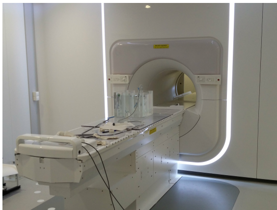
Figure 3.8: The Elekta Unity™ MR Linac device at The Christie hospital in Manchester, UK. The water phantom applied in the present investigation can be seen on the patient couch.
