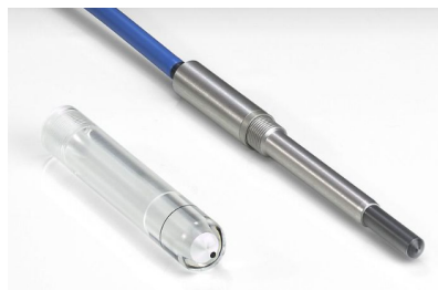
Figure 2.17: A typical Farmer-type IC (PTW 30013) for dosimetry in RT together with a suitable build-up cap (build-up caps can be used for measurements with ICs in air in order to generate more secondary electrons) [PTW-Freiburg].
