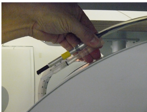
Figure 3.12: The transfer standard IC and the PMMA holder containing an alanine detector. The position on the IC corresponding to the black O-ring on the PMMA holder is marked with the yellow tape.
