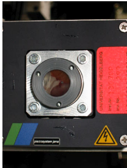
Figure 6.3: The tissue chamber mounted to the translation stage/piezoelectric scanner.
