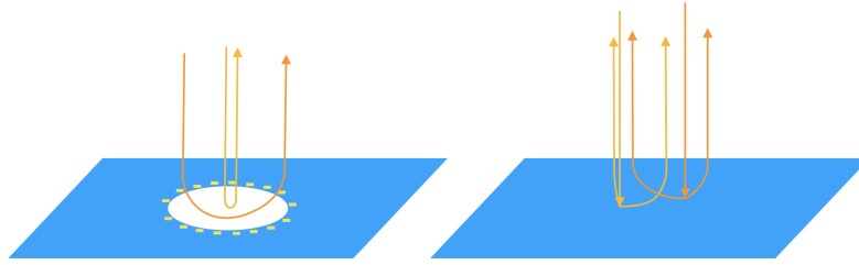
Figure 9.4: Schematic representing the difference of a mirrored beam to scattered. The left side shows the charged defect at which the mirrored beam only takes one trajectory, so all electrons of an image point arrive at one point on the detector system. In contrast, for a scattered beam (right image) all trajectories are possible dependent on scattering angle and energy, so in general electrons from each image point can arrive on the whole detector surface.
