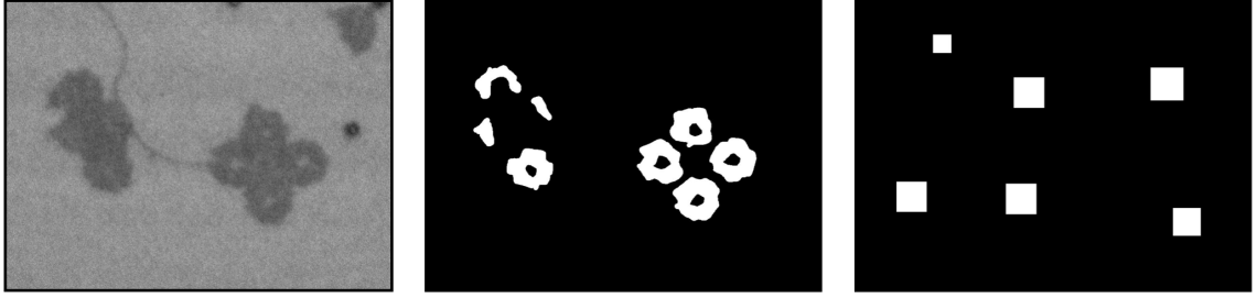
Figure 6.2: Example of manually created masks for further spectrum evaluation from DNA-origami and silicon wafer. Note that the distribution and size of the selected silicon wafer regions is on purpose distributed over the whole image to approximately match the size and distribution of the origamis in order to exclude systematic differences from spectral artifacts (‘anisochromaticity’, see chapter 7).
