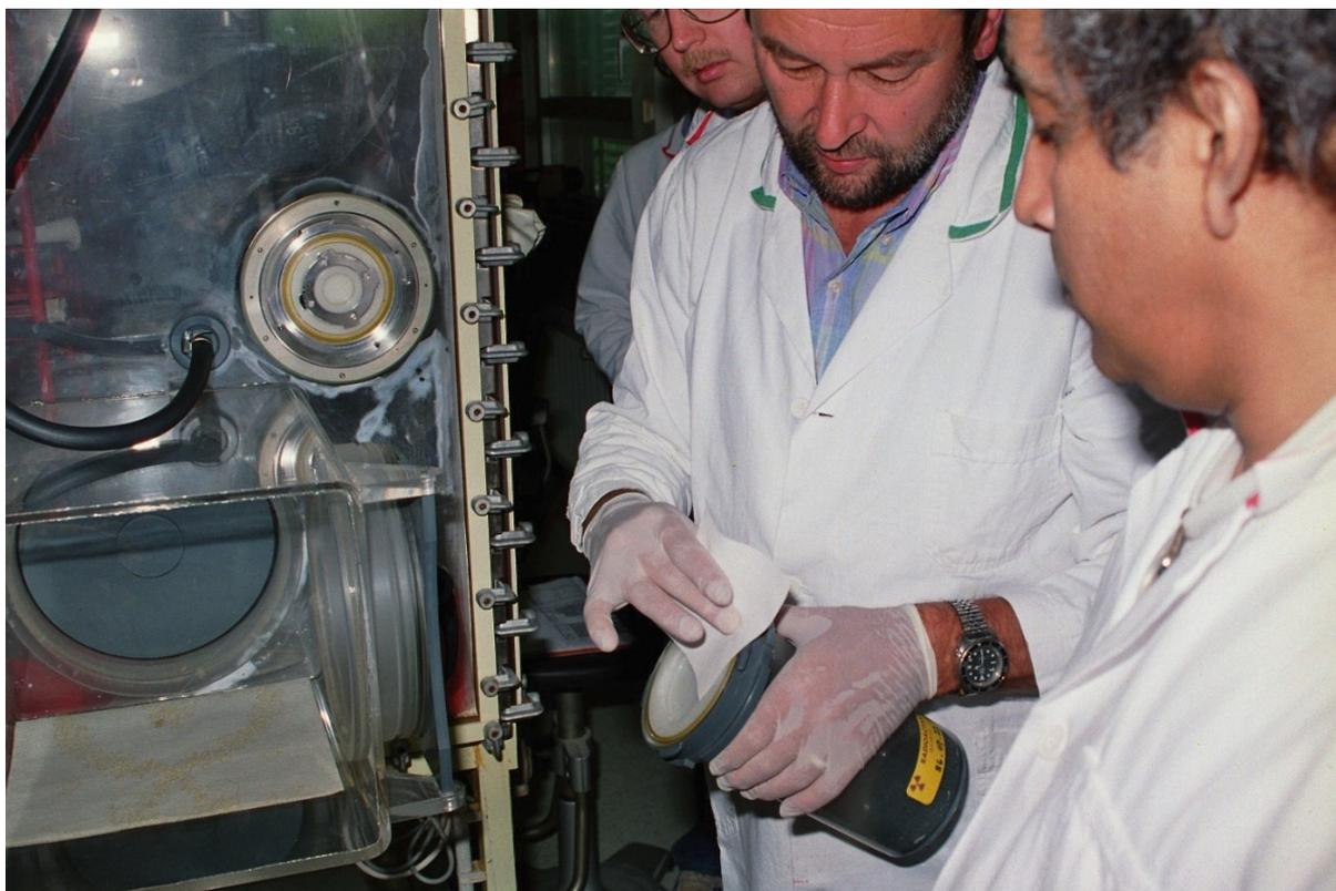
Figure 1: Inspectors taking a swipe sample at a nuclear facility. Photo: IAEA Department of Safeguards, Copyright IAEA, 2016 [9].
