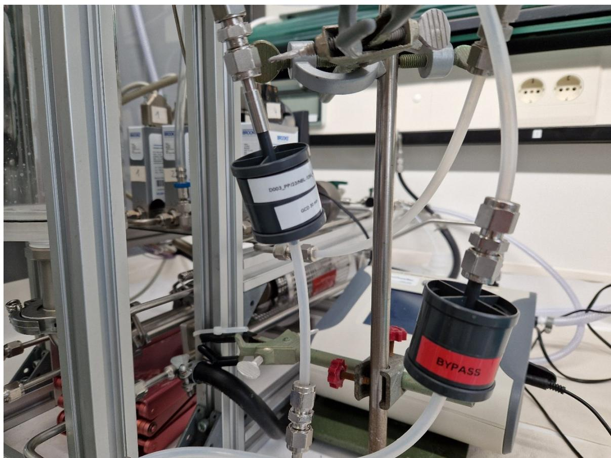
Figure 10: Vacuum impactor containing a substrate (left) within the VOAG setup of the FZJ safeguards laboratories. Bypass for substrate change is on the right.
