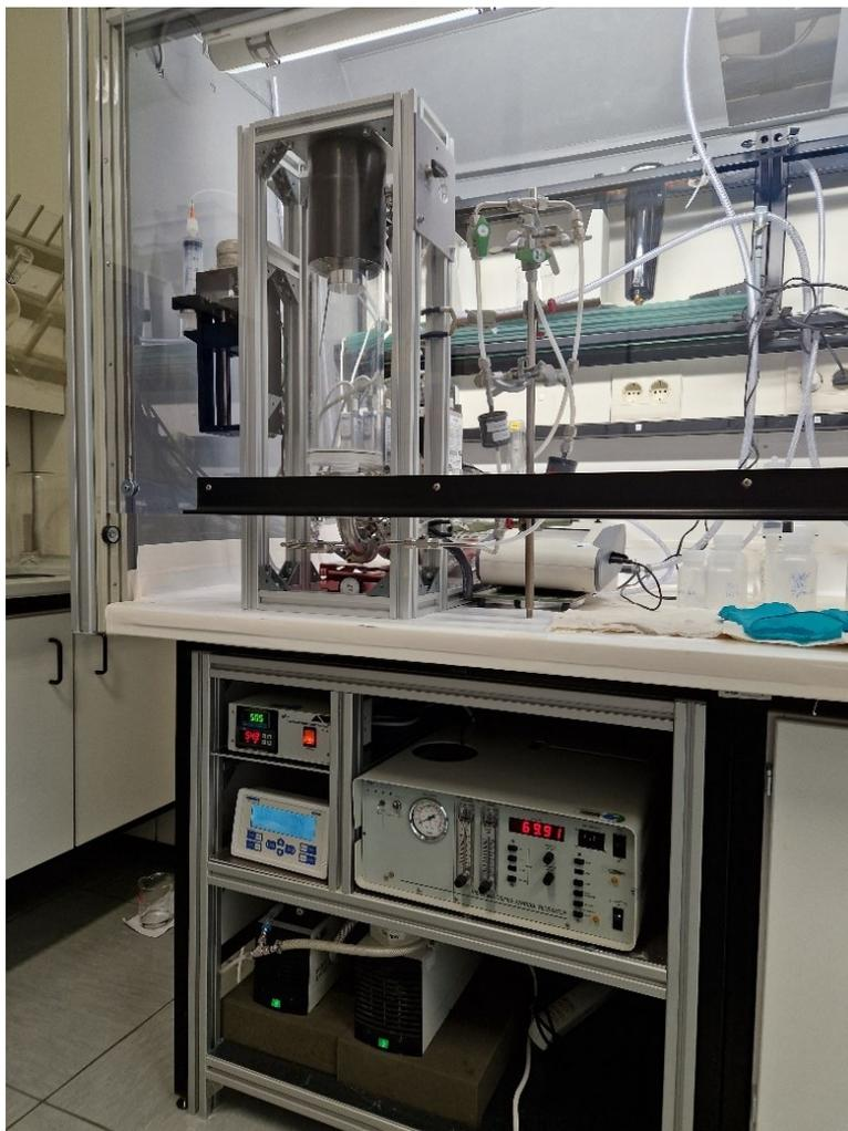
Figure 9: VOAG in the FZJ safeguards laboratories. The syringe with the feeding solution is placed on the top left side, the vacuum impactors with the substrates are on the right side of the drying column.
