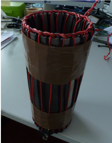
Figure 3.2.8: Left: Used Mu-metal cylinder with its pickup coil (red) and stimulus coil (black), right: measured signals for the determination of the hysteresis loop, note that the current monitor signal was divided by 10 for visualization reasons.
