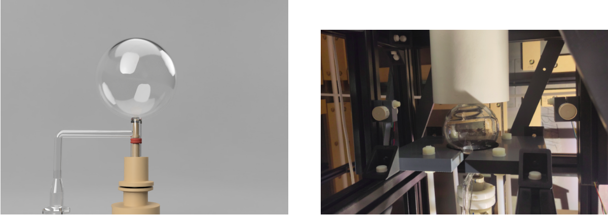
Figure 6.1.3: measurement cell under the SQUID system embedded into the coil system within the MSR. Source: [63].
