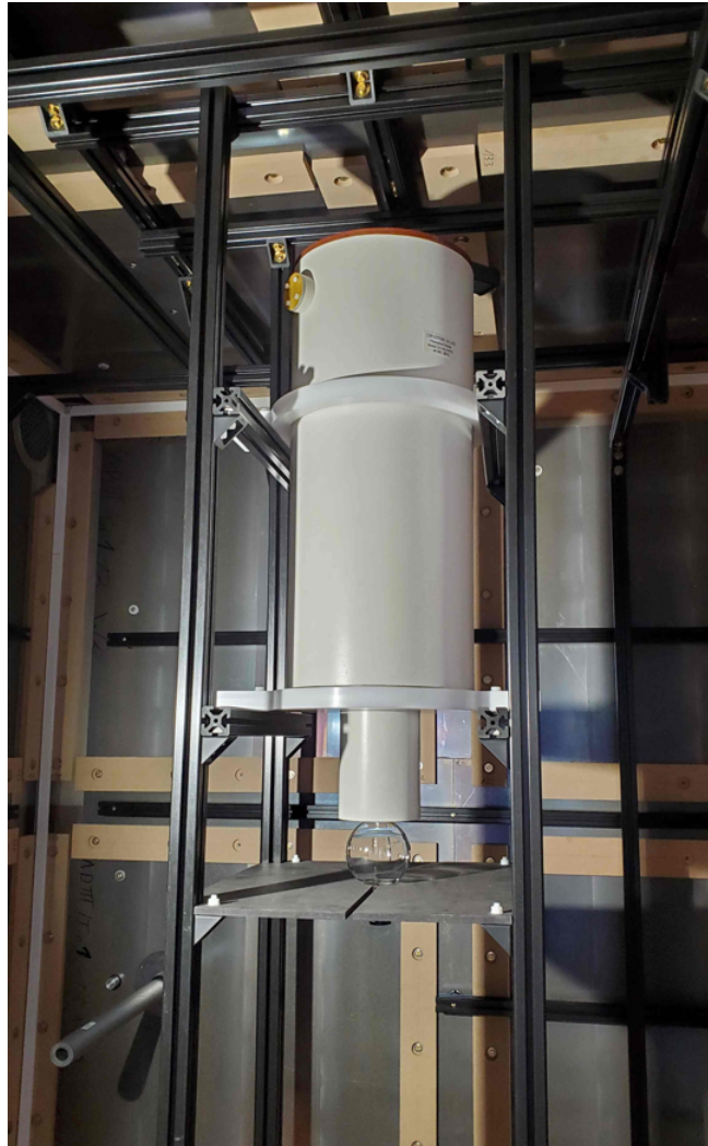
Figure 2.5.3: SQUID system with dewar within the MSR. The measurement cell is mounted below the SQUID at the center of the MSR.
