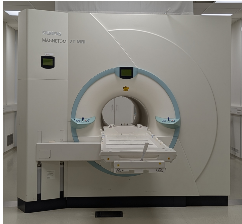
Figure 3.1: 7 T whole-body MR system (MAGNETOM 7T, Siemens Healthineers AG, Erlangen, Germany).
