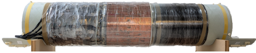
Figure 3.2: Picture of the custom-built 32-channel ^1\text{H} RF coil resting on the bore liner. Here, the setup is shown outside of the scanner bore.
