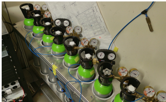
Figure 2.17. Picture of the eight bottles (10 L, 300 b) of radon-free air in the CONUS+ room. The bottles are stored in a rack and connected with pressure reducers to a system of tubes which guide the air inside the shield. A flowmeter (not pictured) is included to check the air flux.
