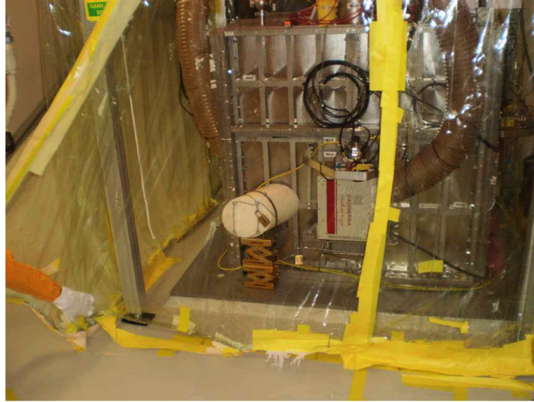
Figure 4.9. Picture of the setup during the californium irradiation campaign of the CONUS experiment at the KBR power plant. The source is contained in the white plastic cylinder. The setup during the irradiation of CONUS+ is the same.
