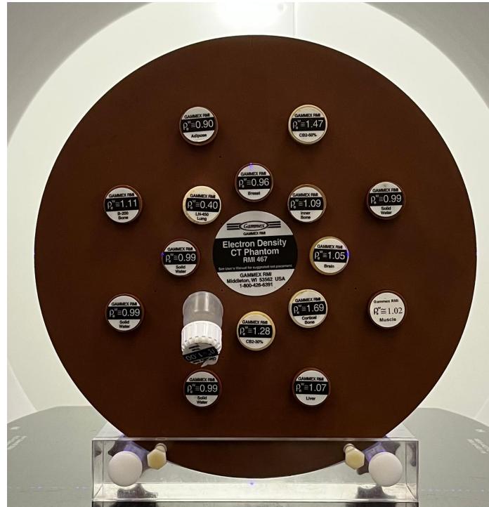
Figure 3.2. Gammex TM RMI-467 phantom (32 cm diameter) used for calibration of the lung region.
