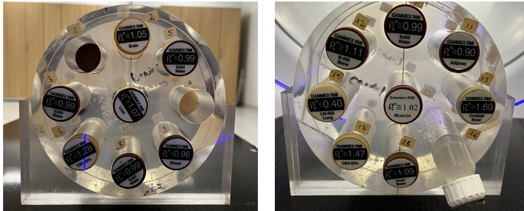
Figure 5.1. Circular acrylic holder (16 cm diameter) with Gammex™ RMI-467 inserts used for calibration of the pelvic region.
