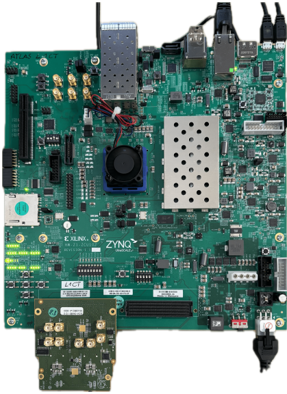
(a) ZCU102 board with FMC.
