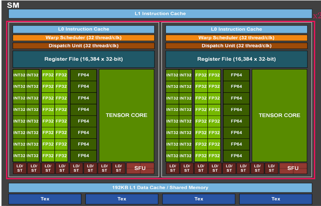
Figure 3.2: Architecture of a Nvidia A100 GPU streaming multiprocessor. The FP64 cores can access a small register for fast storage. Cores within the SMs that are assigned to a block gain access to a shared memory cache for optimised memory access. Figure taken and adapted from [144].
