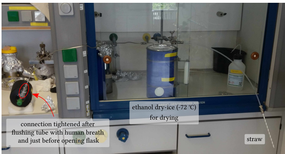
Figure 5.5.: Setup for sampling exhaled human breath. To minimize contamination with unexhaled air, the tube to the flask was flushed with breath before tightening, and just before opening the connection to the flask (left). To dry the sample, an ethanol-dry ice trap located under a laboratory exhaust vent was used (mid). The human breath was blown into the straw (right).
