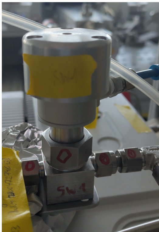
Figure B.3.: The picture shows valve AT SW1 [C8], one of the pneumatically operated globe valves installed. Valves of this type are shown in Figure 3.3 with the symbol \bowtie .
