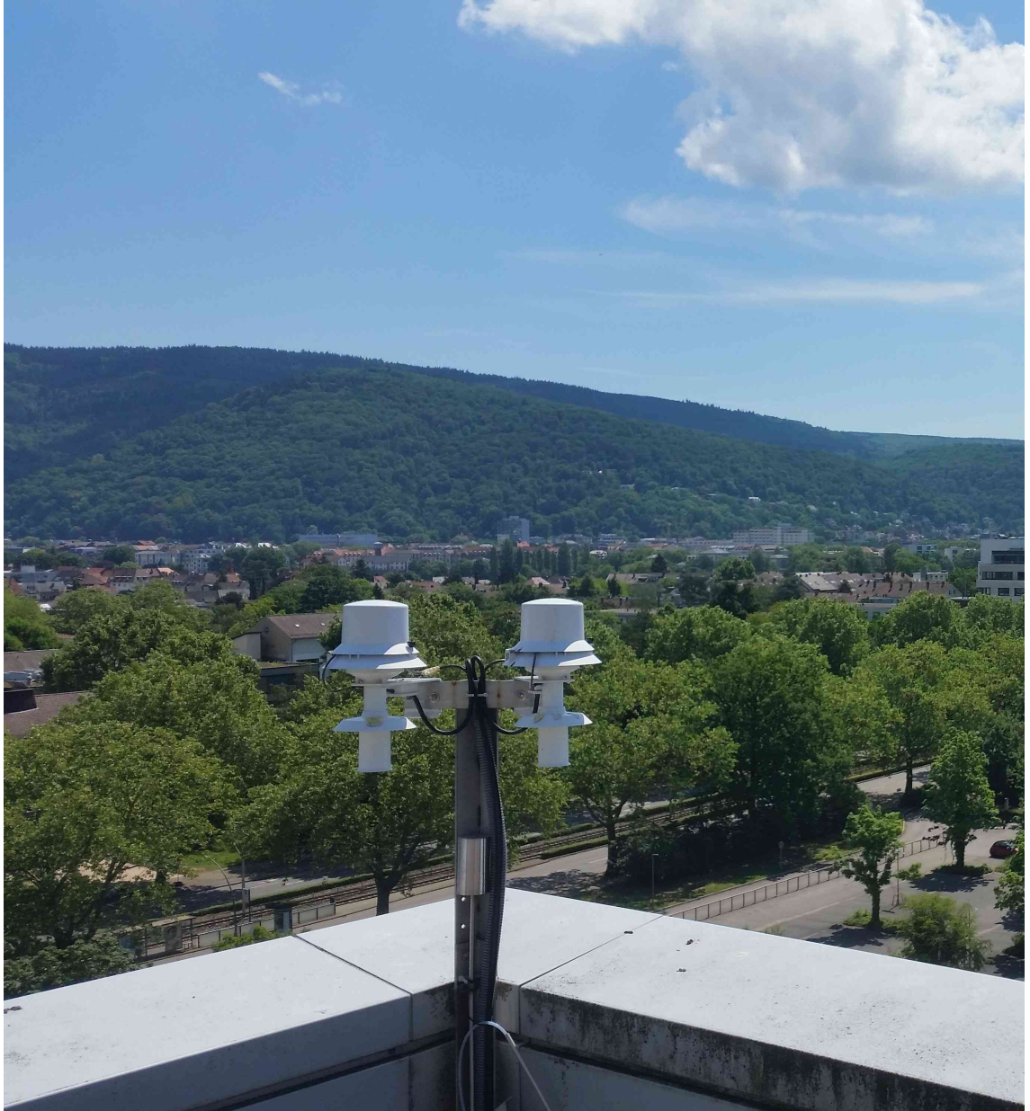
Figure A.2.: Intake for ambient air located at the southeast corner of IUP's roof at approximately 31 m above ground level.
