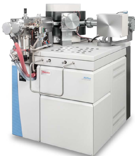
Figure 2.9.: The figure shows the MAT 253+ Isotope-Ratio Mass Spectrometer (IRMS) used. [Image: Thermo Fisher Scientific, 2016]
