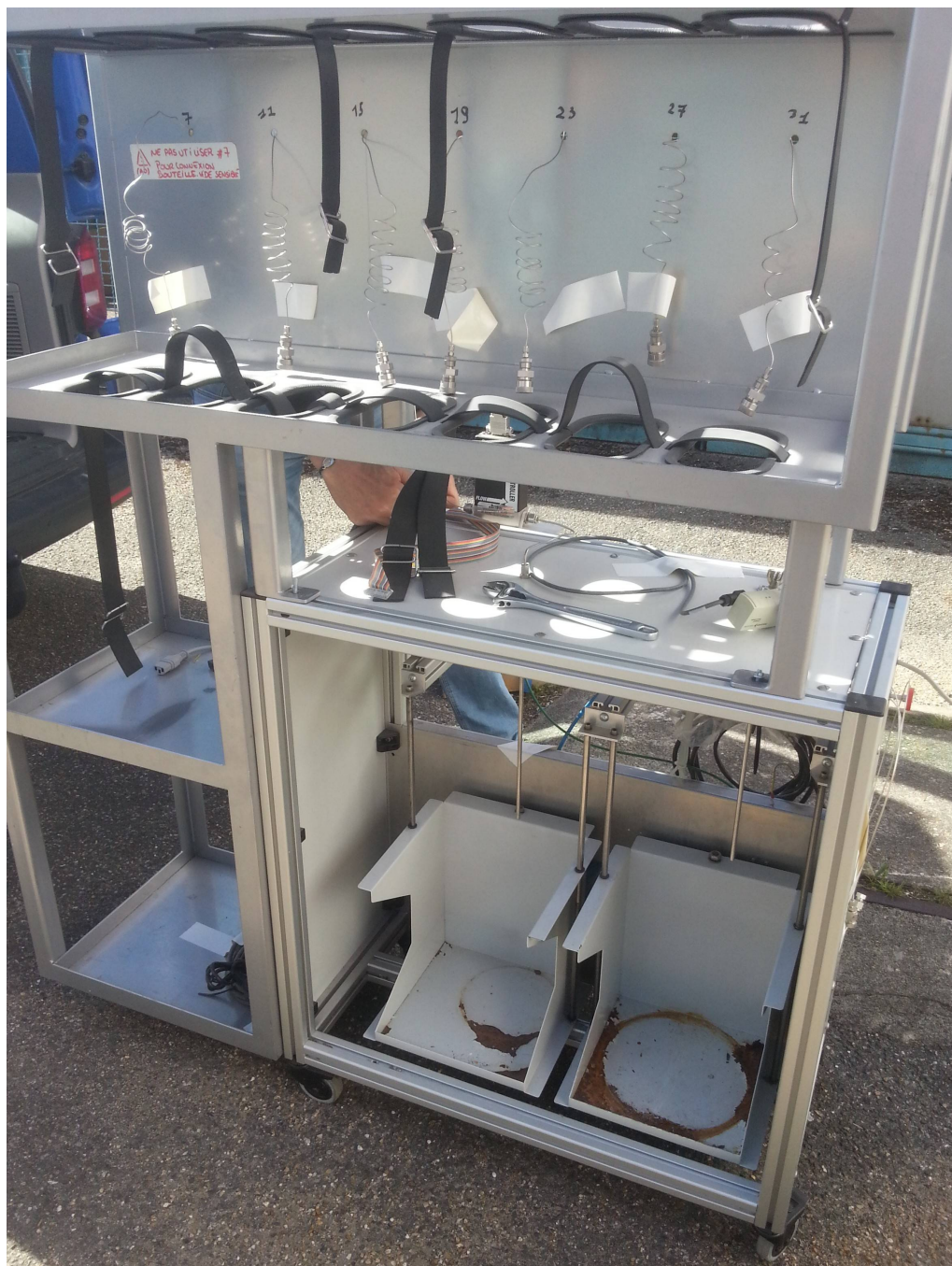
Figure B.20.: The graphic shows the basic structure of the preparation line at the pick-up at the Climate and Environment Sciences Laboratory (LSCE) in France on May 14, 2019. The basic metal frame including two lifting platforms and the connection options for flasks via the multiport valve can be seen.
