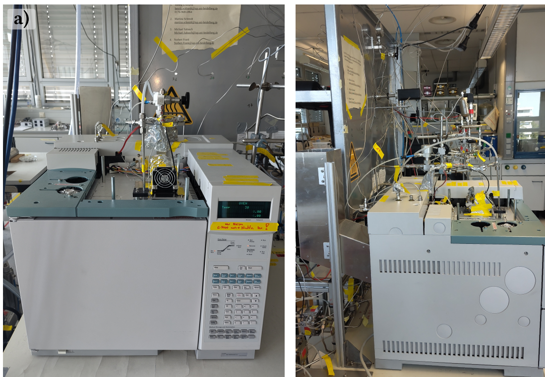
Figure 3.4.: The images show the GC (G1530A, Agilent, Santa Clara, CA, U.S.) a) from the front and b) from the side. In b), the exhaust chimney installed at the end of April 2024 can be seen on the left.
