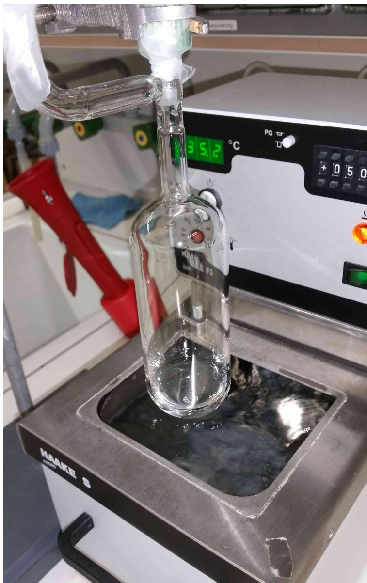
Figure C.1.: This image shows the ~190 mL glass cylinder used as a re-equilibration vessel for producing temperature-equilibrated CO 2 standards. The image also shows the temperature-regulated water bath (F3/S; Haake Fisons) used for re-equilibration.
