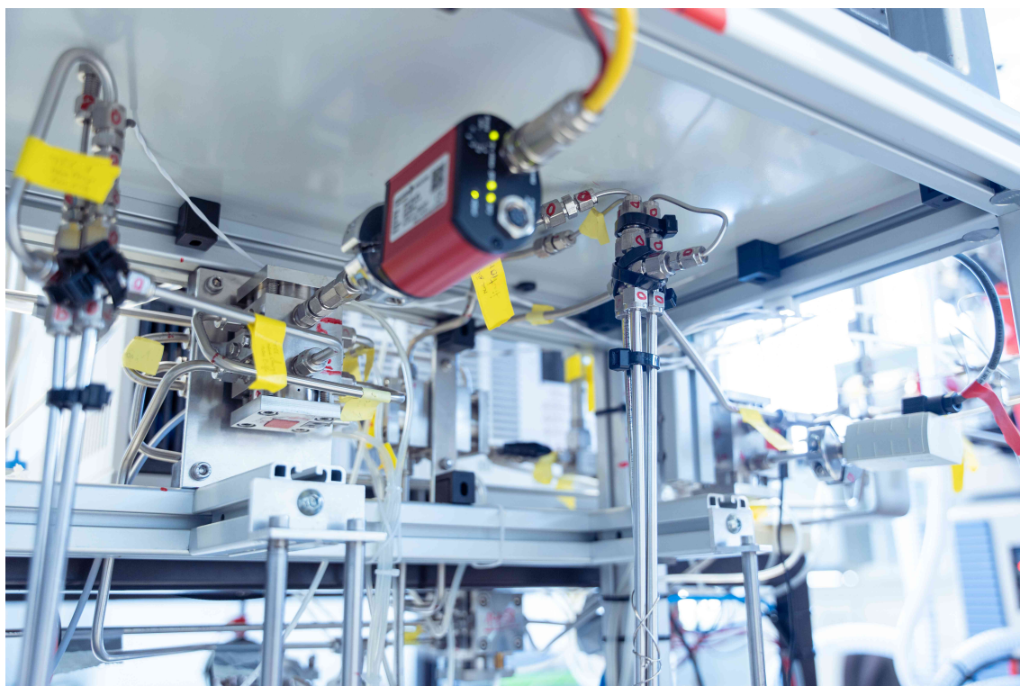
Figure B.1.: The picture shows a close-up example of the basic structure of the Air Trap, including some of the installed stainless steel tubes. In addition to the central pressure sensor RPT [C6], the freezing fingers of the “ \text{CO}_2 trap” [C6-C7] can be seen on the right and those of the “ \text{H}_2\text{O} trap” [D6-E7] on the left.
