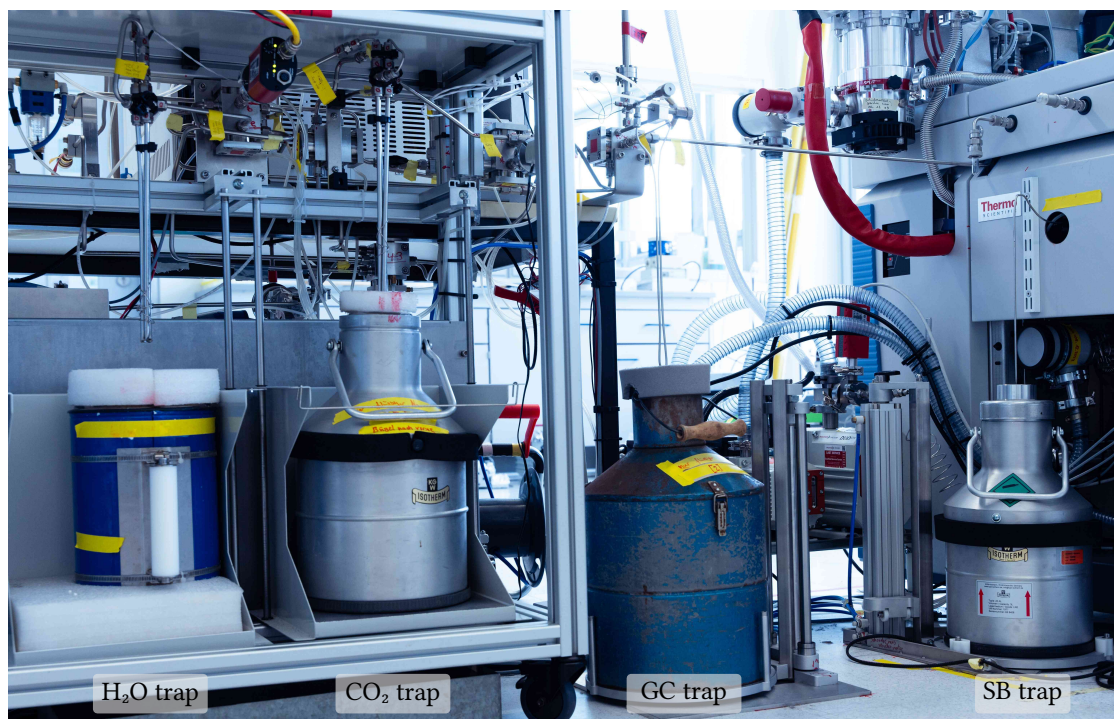
Figure B.6.: The picture shows the four traps of the Air Trap. Dewars are placed on all four pneumatically operated platforms. The \text{H}_2\text{O} trap shown on the left contains a Dewar filled with ethanol dry ice ( -72^\circ\text{C} ). The other three Dewars contain liquid \text{N}_2 ( -196^\circ\text{C} ).
