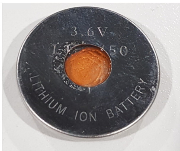
Figure 2.8: Photograph of a coin cell with an optical window, adapted from KIT Campus Transfer GmbH [85].
