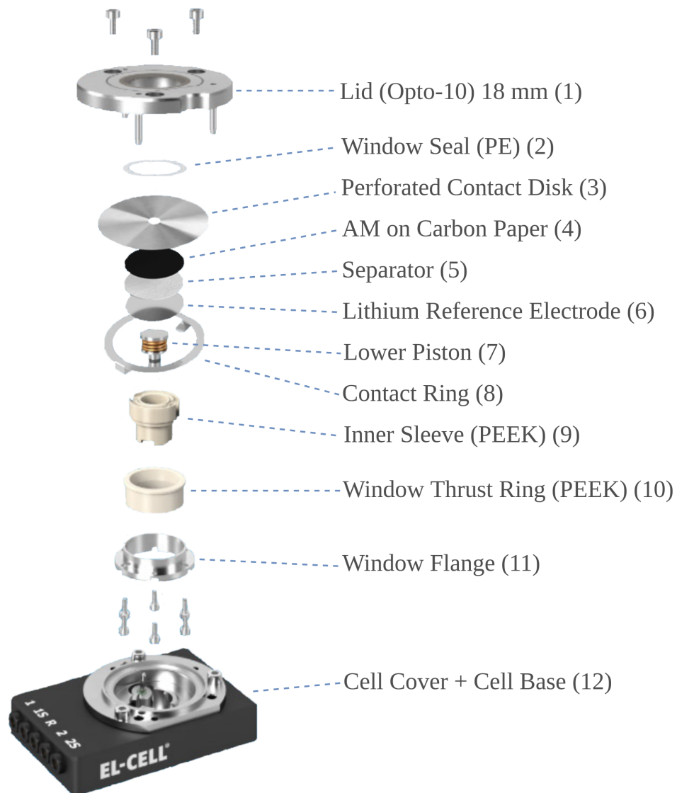
Figure 2.7: Schematic representation of the ECC-Opto-10 cell (EL-Cell) utilized for light-induced electrochemical measurements, highlighting its key components, adapted from [84].
