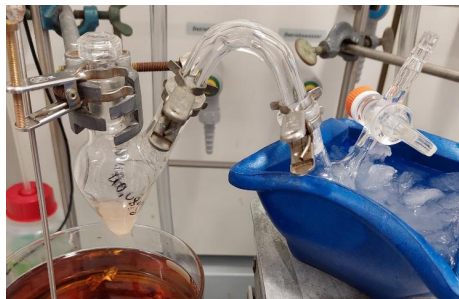
Figure S 10: Setup for the gram-scale depolymerization of pEO with continuous removal of dioxane.
